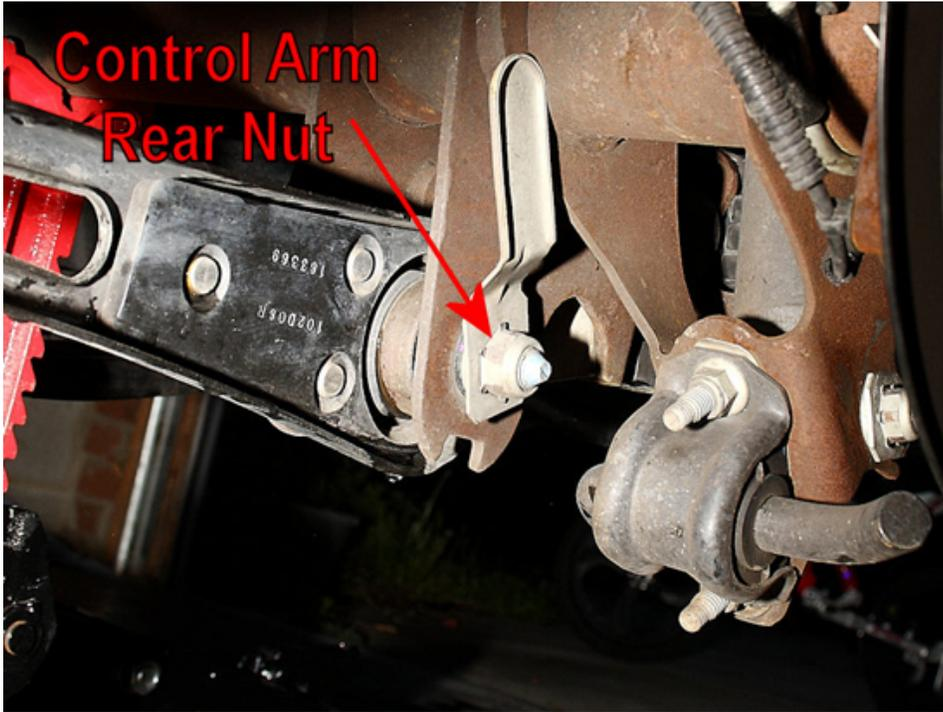
10. When removing the lower suspension arms, make sure to keep it oriented correctly, or note which end is the front and which is the back. The two ends are offset differently, and you must make sure correctly install the new suspension arm in regards to its offset. The rear of the new arm is wider, to match the larger width of the stock arm. This area is offset as well, just like the stock arm. The larger offset should face the middle of the car when it's installed.
