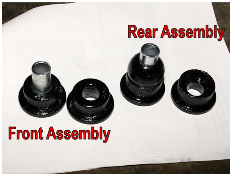
15. You'll also want to apply some grease to the inside of the control arm. Once that's done, press the bushing assembly into place from one side of the control arm. Before pushing the other side's bushing into place, I found it's best to push the steel sleeve halfway out of the installed bushing. This helps to allow air between the bushings to escape, and helps the remaining bushing to seat easier. Once the bushing is in place, you can push the steel sleeve in fully.
