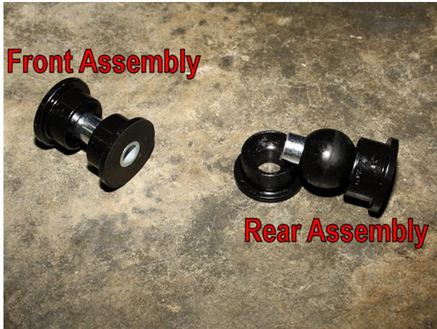
14. Once you know how to assemble the bushings, you'll want to grease them with the supplied grease. Grease the outer portion of the sleeves, and the inner portions of the bushings. Also grease the outside of the bushings with the exception of the bottom that they're resting on in the picture below. The bottom of the bushing will face the suspension mounts on the car, and doesn't really need any lubrication.
