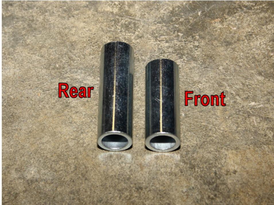
12. You'll also find two different style bushings. Some with a concave face that curves inward, while the others utilize a flat face. The flat-faced bushings are for the front, while the curved ones fit the rear of the suspension arm.
