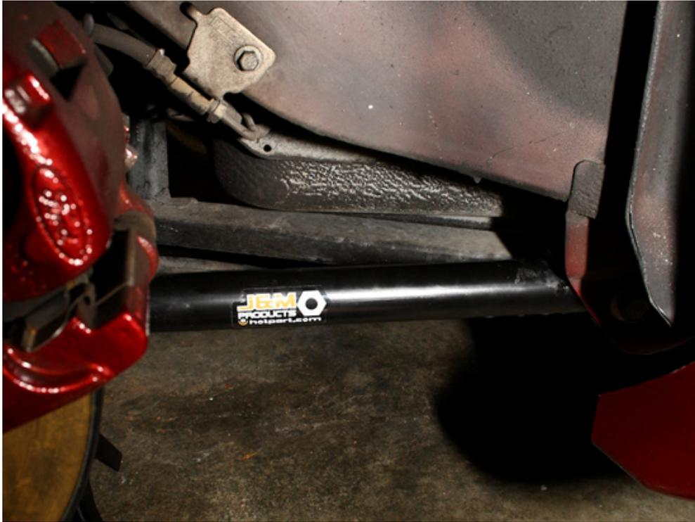
18. The parking brake cable will simply rest on the suspension arm, once you reconnect it to the assembly. You can use a wire tie to hold it in place if you prefer, but it's not necessary.
