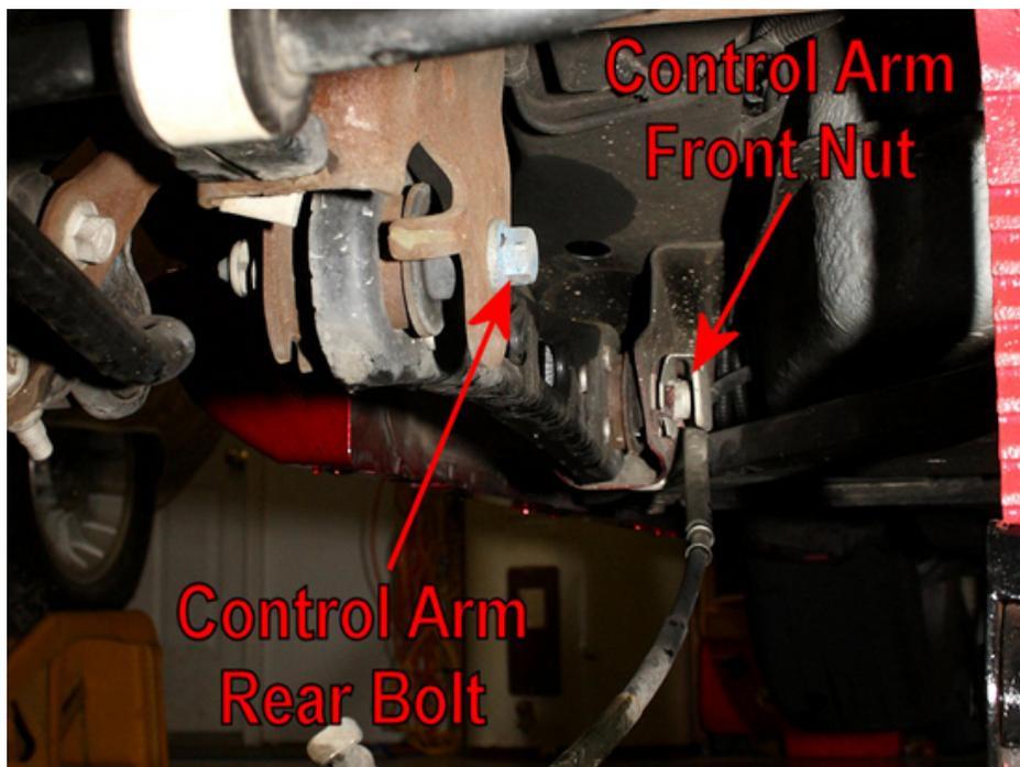
9. As with the front bolt, you don't need to hold the rear bolt's nut to prevent it from spinning. The nut has a tab on it that will catch on the axle, preventing it from turning as you're removing the bolt.
