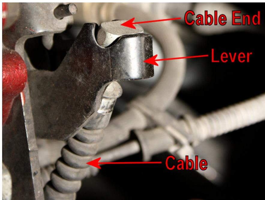
5. Push the lever down, and then twist the cable end slightly to disengage it from the lever. Once the cable end is loose, you can slide the cable away from the lever assembly entirely by pushing the cable down and towards the rear of the car and out of the lever's bracket.
