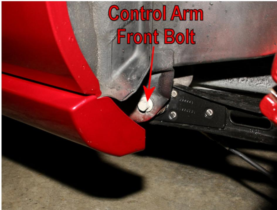
8. Once the front bolt removed, you'll want to do the same with the rear bolt. Again, an 18mm socket and socket wrench needs to be used.
