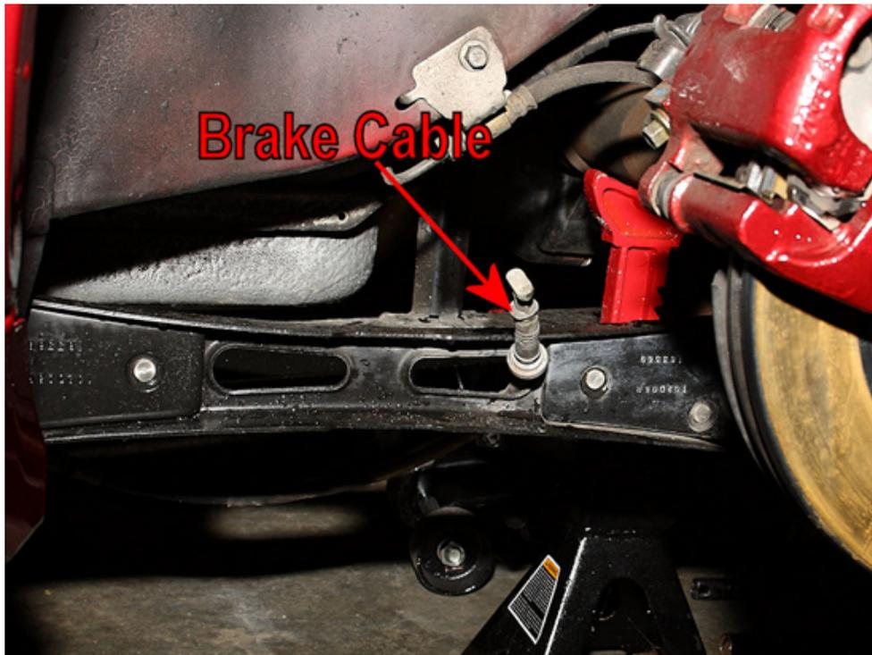
7. Once the parking brake cable is free of the lower control arm, you're ready to begin the actual removal of the arm itself. Using an 18mm socket and socket wrench, loosen and remove the front control arm bolt. The rear nut is clipped, preventing it from turning, so there's no need to hold it with a wrench. Make sure to keep the front and rear bolts separate and don't mix them up, as they are different.
