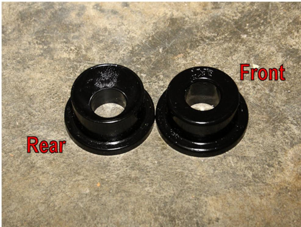
13. Get familiar with how the various parts fit together before you grease and install them. The rear of the arms will use the polyurethane bushing balls nestled between the curved rear bushings. A long sleeve passes through all of the components. The fronts of the arms use the shorter steel sleeve and the flat-faced bushings. When installed, the bushings will be pushed together, but I've left them separated for clarity purposes in the picture below.
