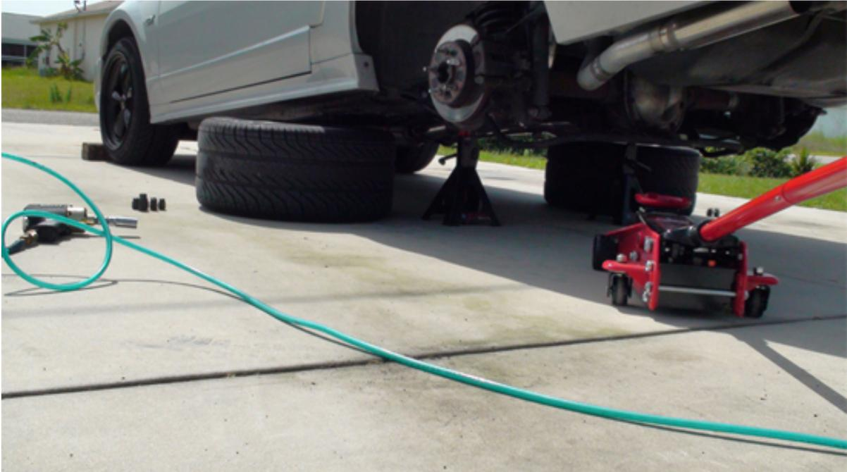
3. After making sure that the car is safe and secure use your 18mm wrench and your ratchet with the 18mm socket (I used an impact wrench which made it very easy) to loosen the 2 18mm nuts and bolts. (I started on the passenger side of the car)
