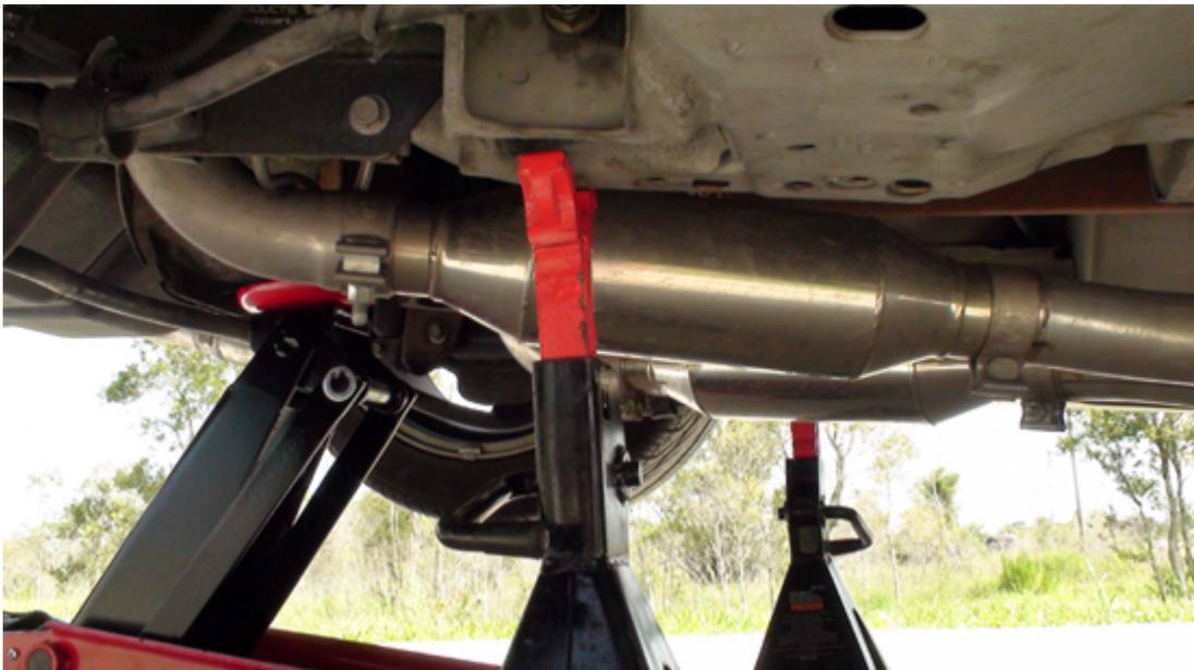
2. Take the rear wheels off and place under the body rails for safety
