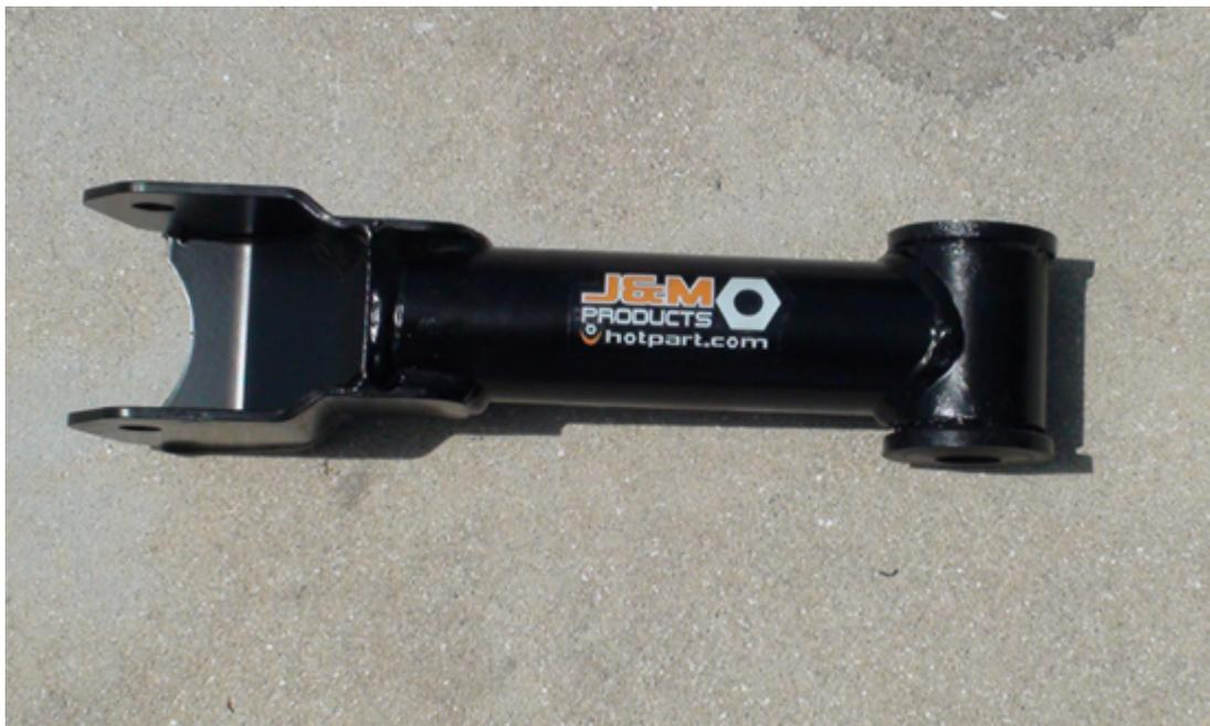
8. Next line up the holes of the bushings you just installed with the holes on the upper control arm mounting bracket that is on the body of the car. Make sure the J&M lettering is facing the ground. Slide the bolt through and put the nut on but don't tighten it yet. Rotate the upper control arm down and line up the boltholes for the rear end attachment. This should be easy as long as you didn't change the jack position. Slide that bolt in replace the nut and now tighten everything down.
