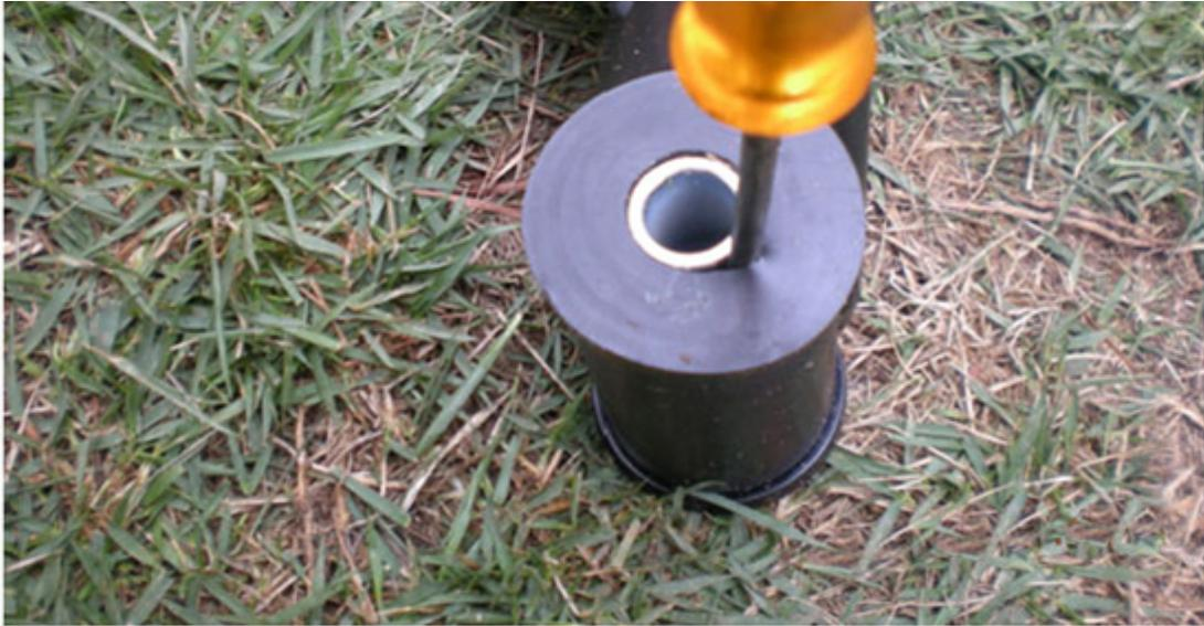
7. Stick a small screwdriver between the sleeve and the bushing, push in 2 inches and gently pry up. You will hear air escaping. Push the bushing in further and repeat these steps for both sides of bushings, until they become flush. Take your time and be patient it will go flush (thanks Jeremiah Campbell for that information).
