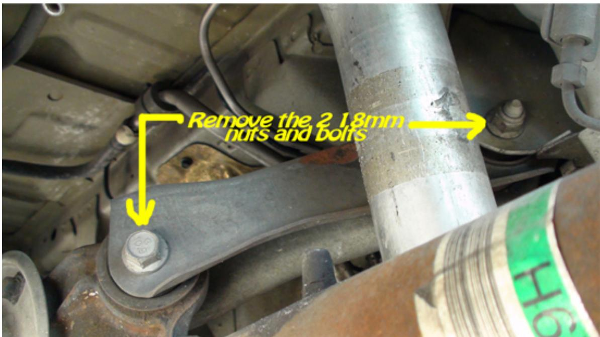
4. Once the nuts are off, to get the bolts out I used my jack to raise the rear end very slightly to take the tension off while pulling on the bolt that connects the upper arm to the rear end. You should feel it get loose, stop jacking and pull the bolt straight out. Now that the lower bolt is out the top bolt will come out real easy.
