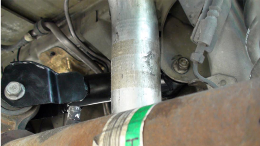
10. The driver's side is no different. Loosen the 2 18mm nuts and bolts just like the driver side. The only difference at least for my car is the bolt that mounts the control arm to the body is kind of tough to get at. This is where the swivel socket and 4" extension comes in handy.
