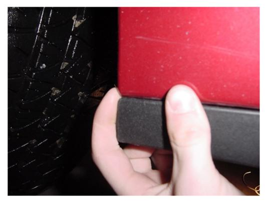
6. Next, locate the first hole on the corner of the spoiler. Using a drill, drill the hole out so that the bolt can be fastened. Only drill far enough into the fascia until the drill bit pokes through the inside of the fascia. (I used a 1/2 inch drill bit for my personal bolts. The fasteners that come with the kit use a 1/4 inch drill bit).
