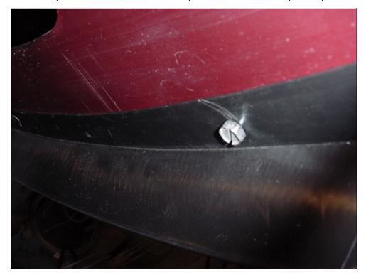
11. If installed correctly with bolts, there will be plenty of room inside the fascia for tightening of the nut and lock washers. The picture below shows the inside of the fascia with part of the spoiler installed.
