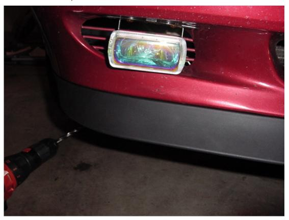
9. After drilling the hole, insert the fastener and screw in the fastener insert tightening the fastener. The fasteners are strong, but to stop any un-needed stress on the fasteners and the spoiler, use something to prop the spoiler up so it is not simply dangling from the car.
