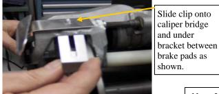
Bend clip in or out for adjustment to fit as needed.
