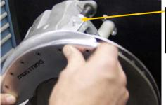
Bridge should rest on caliper
