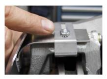
5. Tighten with wrench about a <sup>1</sup>/<sub>4</sub> Turn or torque at 25 inch pounds. **Do not over tighten.**
