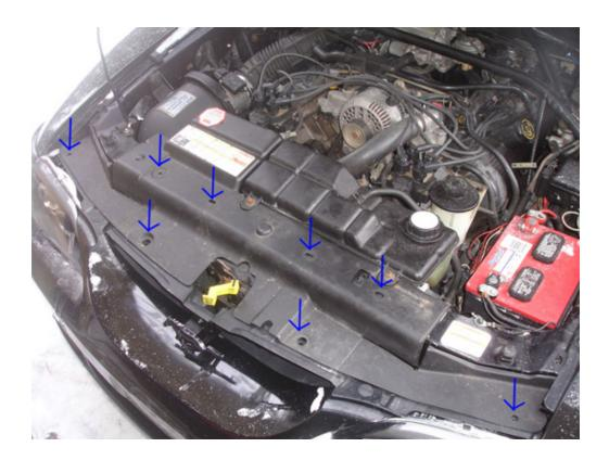
4. Next, take off the coolant reservoir by removing the three, 10mm nuts.
