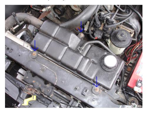
5. Now pull the coolant reservoir up off the bolts, and pull the overflow tube up and over the cap so it is out of the way. Then twist the passenger side of the tank to the front of the car and push the whole assembly to the driver's side of the car so it is out of the way.
