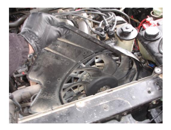
8. Here you can see the difference of the new Mishimoto fan compared to the stock fan with shroud. Even though it is smaller with no shroud, it still performs excellent.
