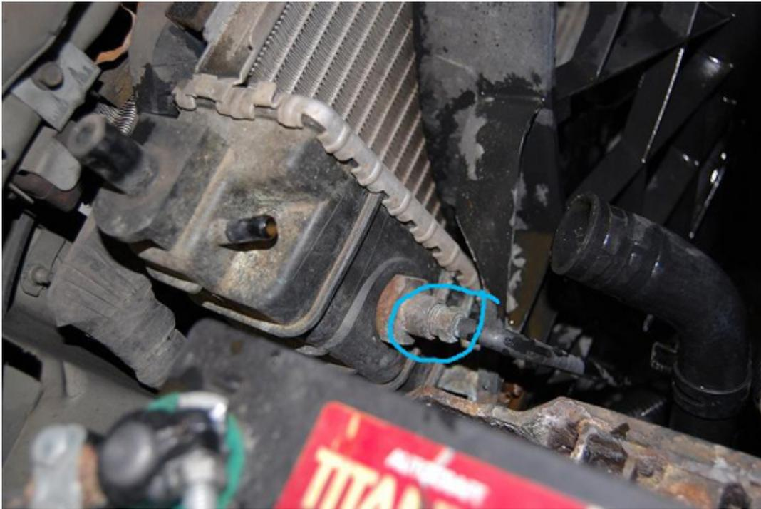
6. At this point, you want to close the drain on the right side of the radiator and move your drain pan to the left side placing it under the lower radiator hose. Using your 13mm or 1/2" wrench, remove the two transmission lines that connect to the left/driver side of the radiator and the lower radiator hose. The radiator/fan assembly should now lift right out together; it may take a little wiggling.
