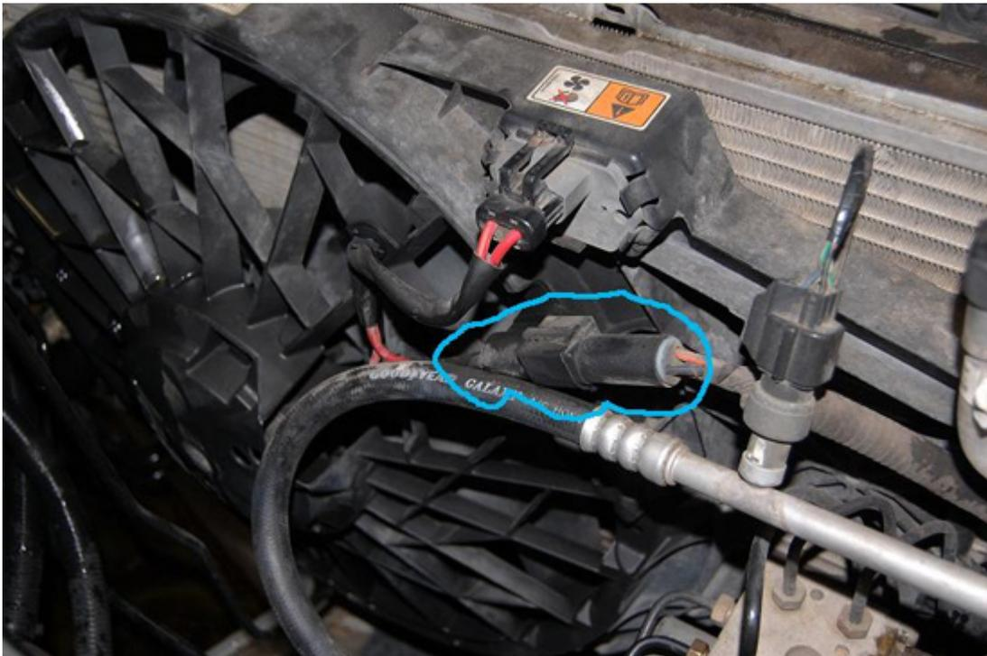
5. Unplug the fan. This is where the miniature pick comes in handy to lift up the tabs on the plug. There is a tab on the top and bottom side.
