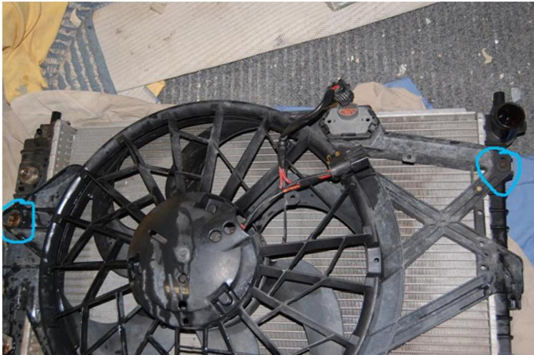
7. Remove the two, 8mm bolts holding the fan assembly to the radiator and slide the fan assembly towards the top of the radiator to slip it out of its mounting slots. At this point, if you have a bunch of junk in the overflow tank fill it with 1/3 the bottle of flush and hot water shake it up and drain, repeat this until the tank is clean.
