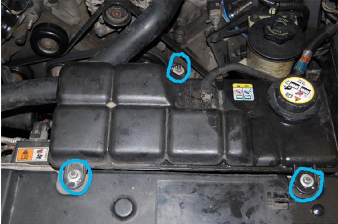
2. Once the radiator has drained, remove the three, 11mm nuts holding the overflow tank to the car which are circled in the picture above. Remove the hose on the bottom side of the overflow tank and the smaller diameter hose connected to the top of the overflow tank, where it connects to the radiator.
