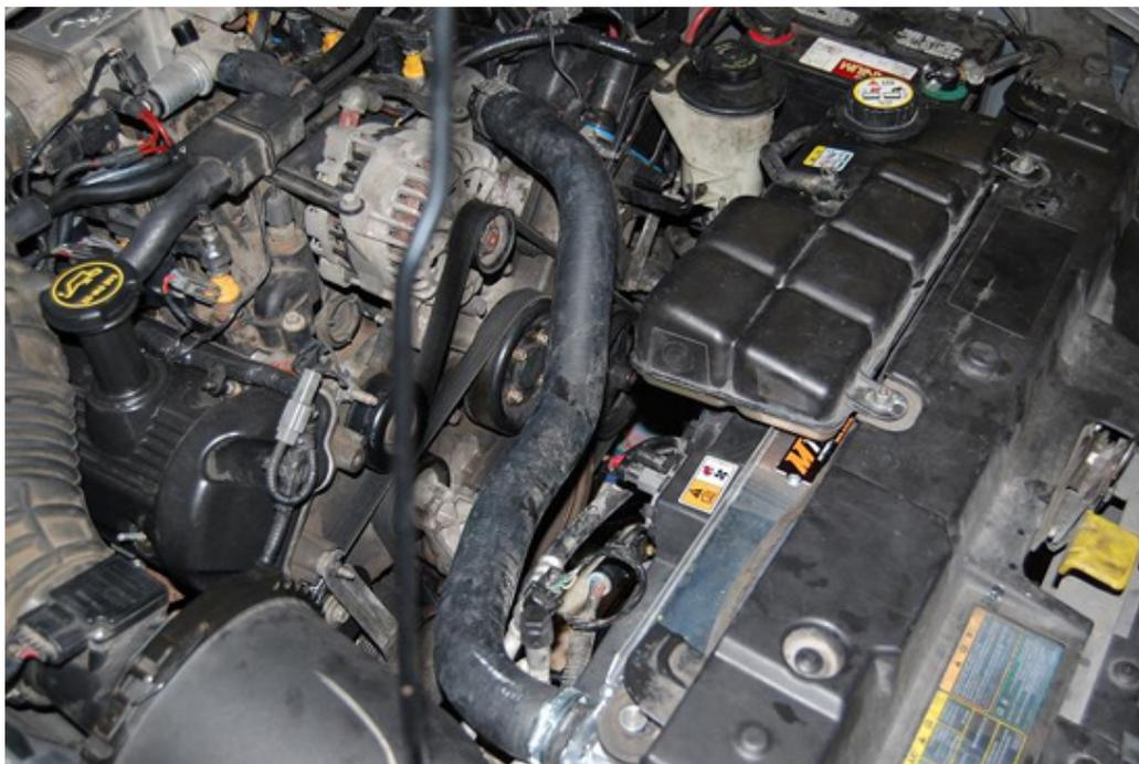
12. Connect the overflow tank to the larger diameter hose and then slip it over the 3 mounting studs. Install the three, 11mm nuts and connect the smaller diameter hose to the radiator.
