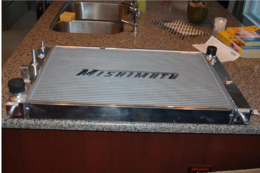
9. After unpacking the radiator, remove the drain cock, inlet/outlet caps, and transmission line plugs. Once removed, place the radiator in the car, making sure the dowels on the bottom go into the rubber mounts. Reach under the right/passenger side of the car and reinstall the drain cock.
