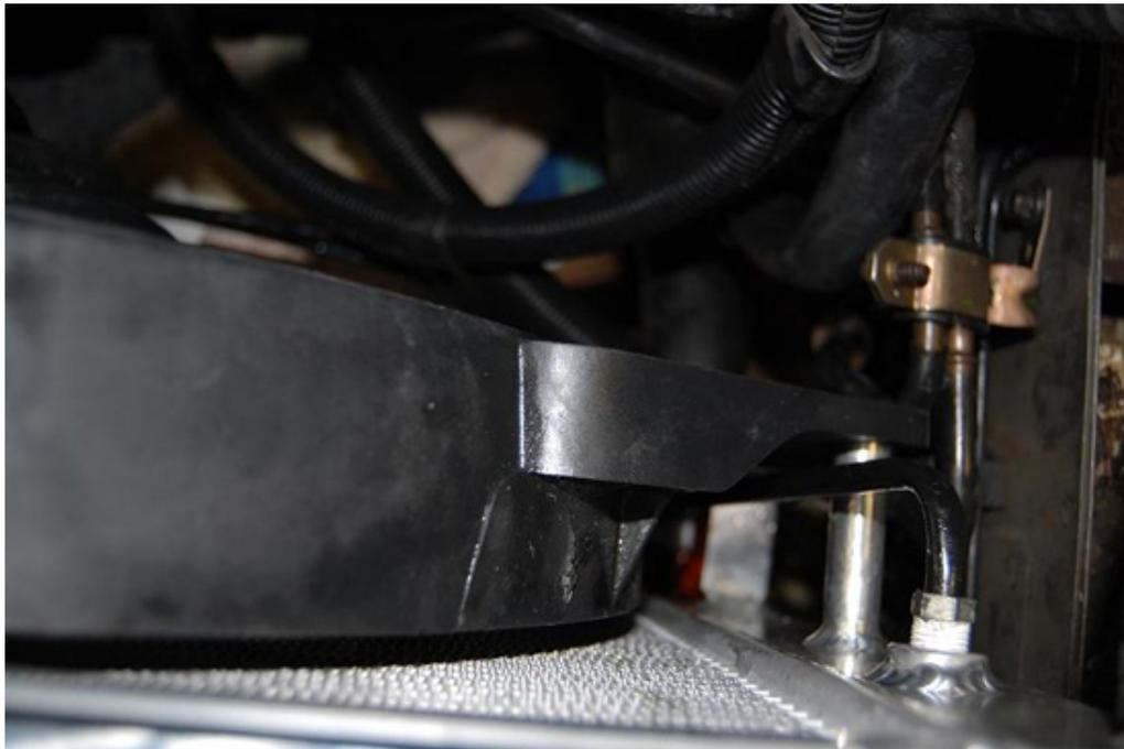
10. Put a little Teflon tape on the transmission line threads, making sure to start the tape a few threads back from the edge so it does not get into the radiator (if you decided to use Teflon tape) and thread the lines into the radiator using the 13mm or 1/2" wrench. You do need to get them fairly snug so they do not leak. In the picture above, you can see how the line runs between the fan assembly and radiator.
