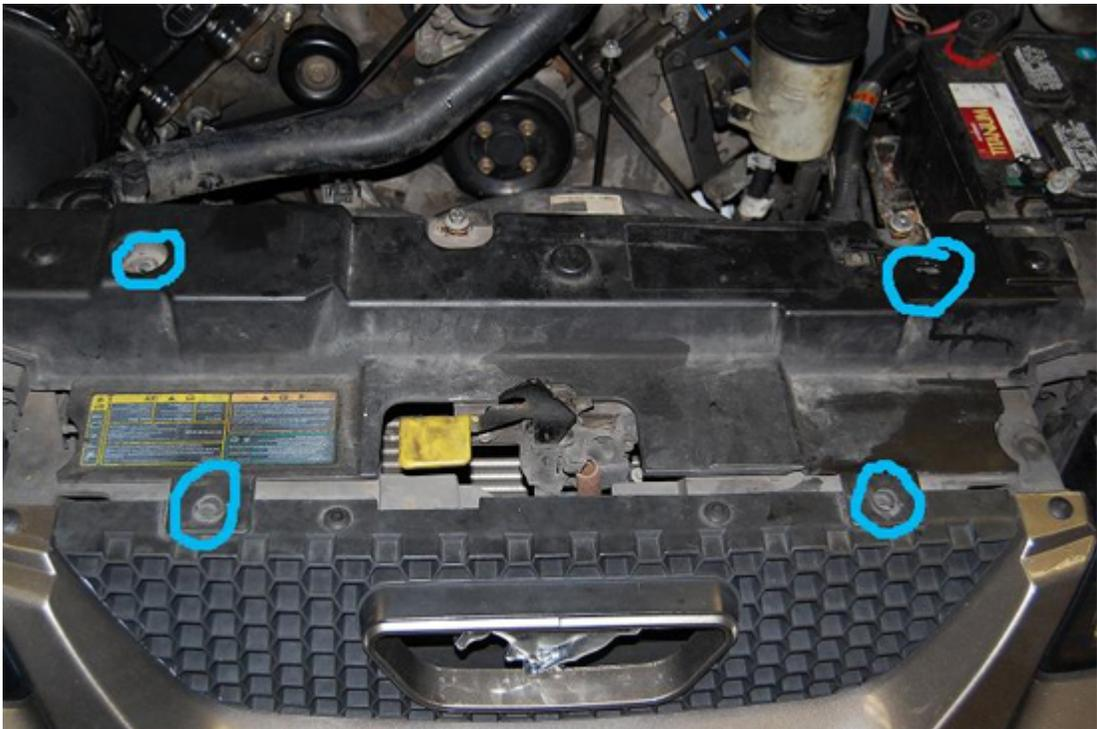
3. Remove the 4 plastic push-in clips that hold the plastic radiator cover on and remove the cover.
