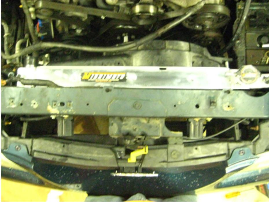
11. Reattach the lower radiator hose. Reattach the upper mounting brackets, and finally reattach the overflow tank, overflow tank wiring harness, and computer unit harness by tightening its bolt with the 3/16 socket. Finally reconnect the fan's harness as well as the two harnesses you removed from the fan shroud in the beginning. Double check all harnesses have been reconnected, all brackets are tight, and nothing is obstructing the pulleys.
