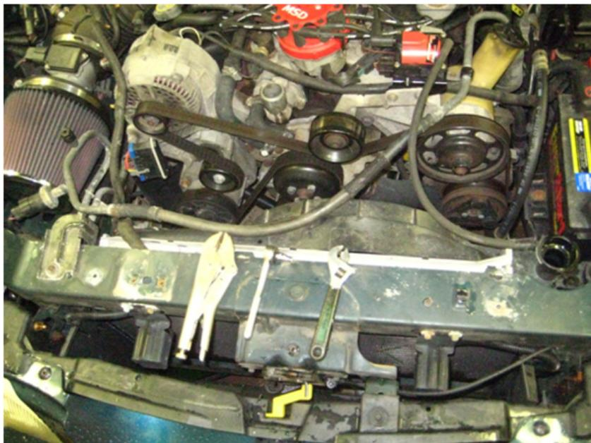
6. Now remove the upper radiator supports. One is on the passenger side as well as the driver's side. The bolts can be removed with the 5/16 socket, and simply pull up on the brackets to remove them from the radiator and the car itself.
