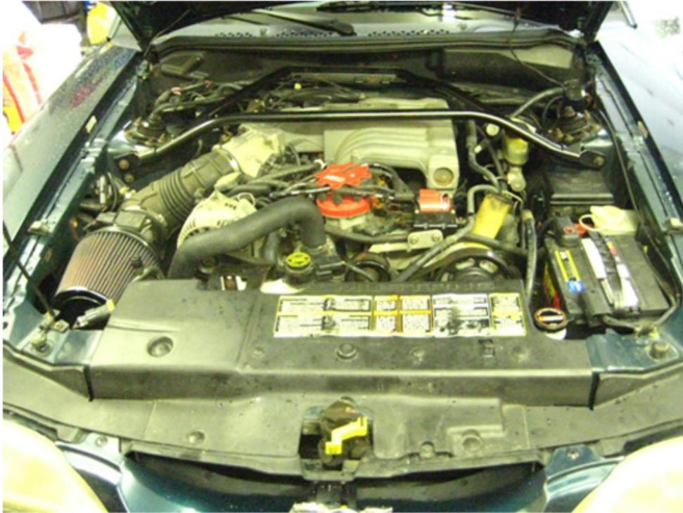
14. Remove the radiator cap from the new radiator and start to pour in "your specific" coolant mixture. Fill until the fluid level reaches the top. The radiator will take more fluid since the radiator is now bigger than the stock unit was.
