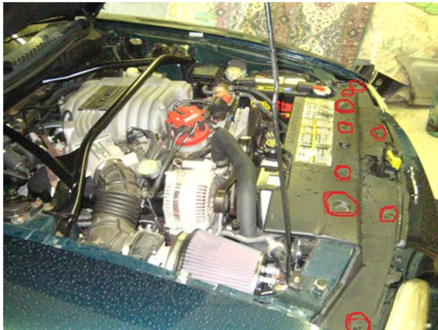
4. After removing the 8 plastic pushpins you can now lift the radiator shroud off the car and set aside.
