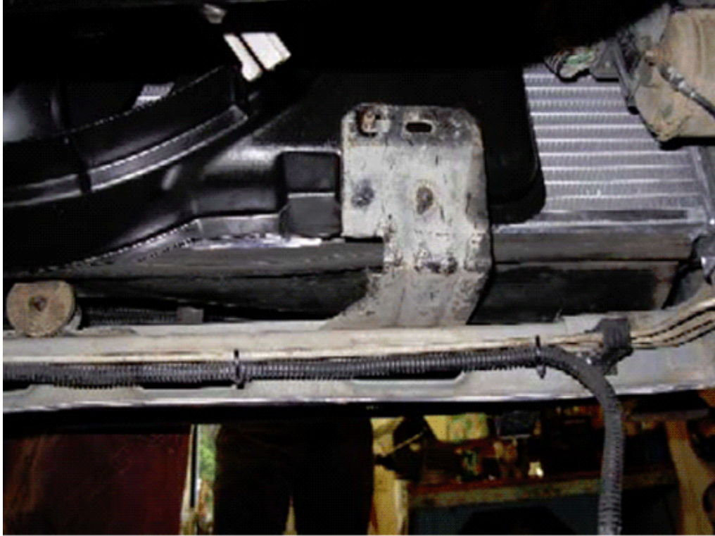
Lower passenger side bracket. Notice that the fan shroud is behind it.
