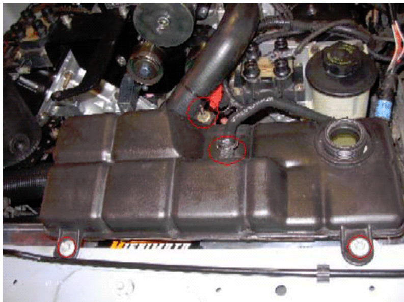
Mounting studs, rod, and overflow tube circled in red.
