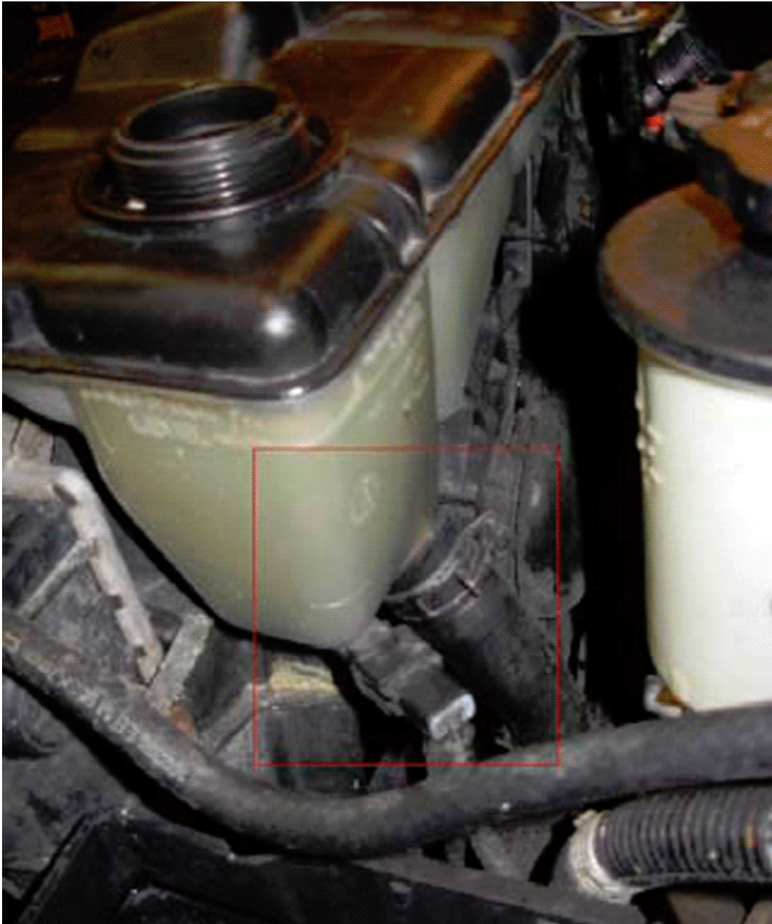
Coolant reservoir with level sensor and tube outlined in red.
