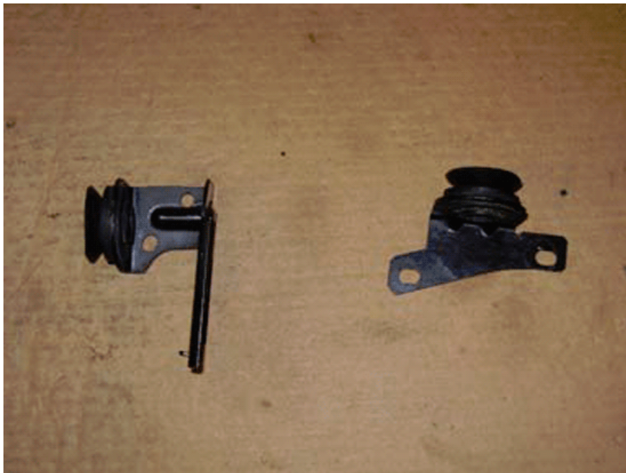
Upper radiator mounting brackets.
