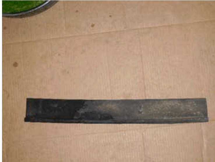
Rubber debris deflector.
