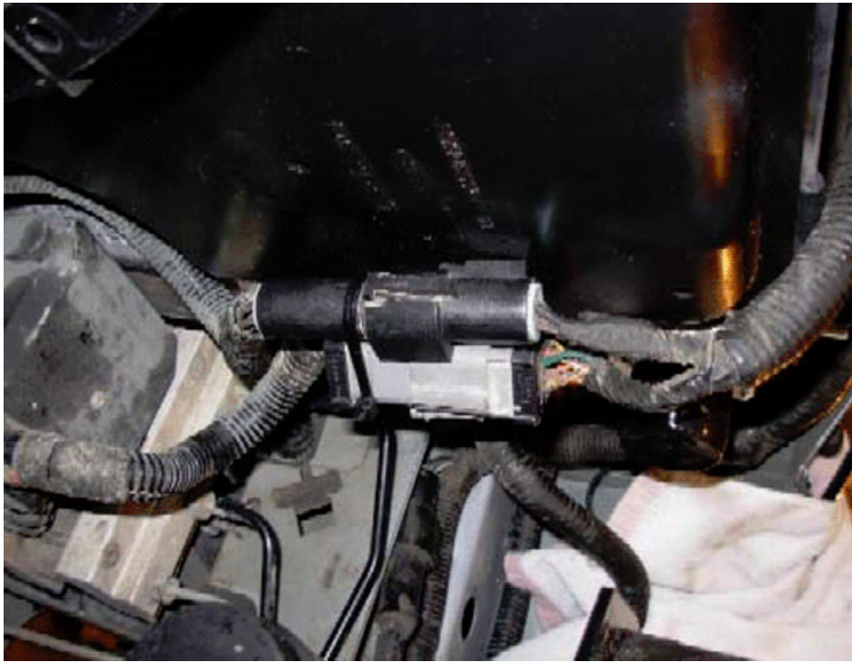
ABS connectors zippered together.
