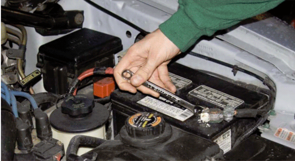
Removal of the negative battery terminal cable.
