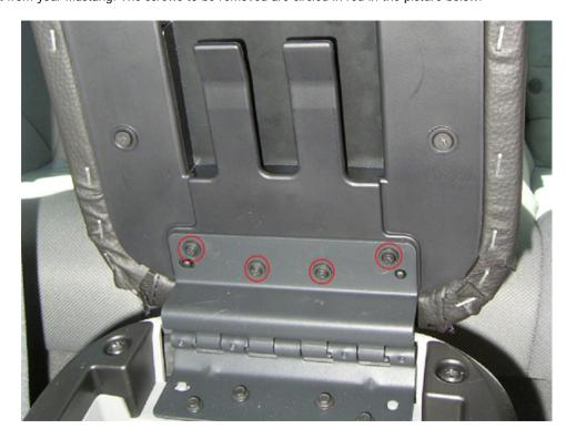
2. After removing the arm rest from your Mustang, place it on a flat table. You will now have to remove the inner plastic casing so that your arm rest cover will be able to have a nice seal and give off that professional look to it. Below is a picture of the plastic casing along with the six screws that need to be removed, using the Phillips screwdriver. The screws that need to be removed are circled in bright green.
