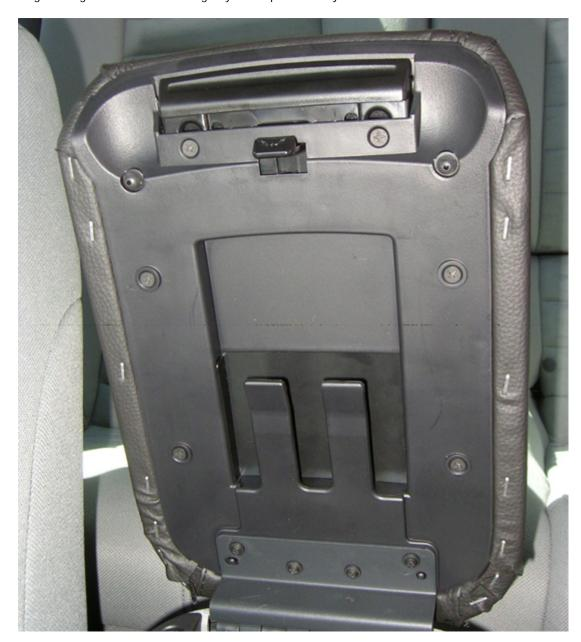
10. After all of your edges are stapled and secured to the existing arm rest, put the plastic covering back on and screw into place. Because of those holes we had made in the beginning, the plastic covering will go on very easily.
