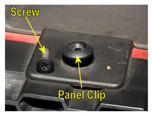
3. With the screws and clips removed, pull the radiator cover off and set it aside.
