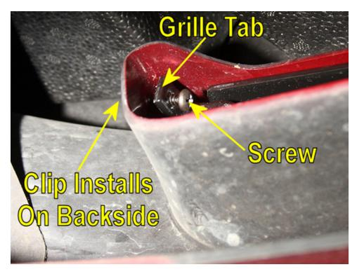
12. To tighten the screws, a long screwdriver passed through the front of the grille is an easier method than trying to tighten the screws up from the backside of the bumper cover.
