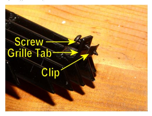
11. Place the grille into the car's bumper cover, and thread the screws on each end down into the metal clips. The clips will go on the backside of the bumper cover. This step is easiest accomplished while under the car, which is why the car was raised earlier.
