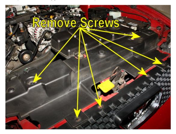
2. The screws are plastic, and sit inside a recessed washer-like clip. Once the screw is removed, you can pry the clip straight up with a flathead screwdriver. As the screws and clips age, you may find that the screw simply turns without coming out. If this occurs, use a small flathead screwdriver to pry the screw up as you're turning it. This should allow the threads on the screw to grip and then screw out of the washer-like clip.
