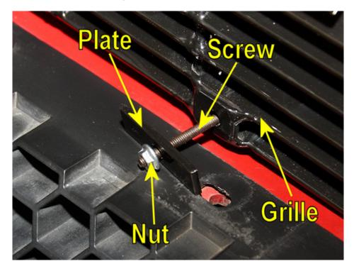
6. Once the grille is positioned against the front of the factory grille, install the supplied hardware to hold it into place. All you need to use to tighten the screws down, from the front, is a Philips head screwdriver. You can easily prevent the nut on the backside of the grille from turning with your fingers. Once completed, reinstall the radiator cover and factory fasteners you removed earlier.
