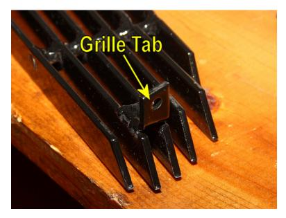
9. Position the grill in place, and then mark the spot for the holes you'll drill. I used a punch, but you could just as easily use a Sharpie permanent marker or similar marking tool. Then use a drill bit, an 1/8 inch bit works well, to drill holes for the screws.
