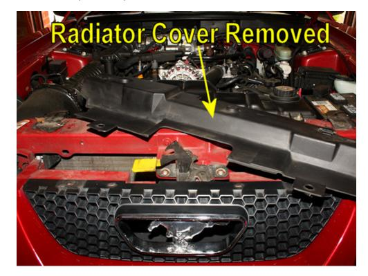
4. There are two more screw and clips on each side of the grille. Remove them, just as you did the others. Once removed, you can flex the factory grille away from the car allowing you access to the area behind the factory grille.
