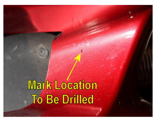
10. When installing, the screws will pass through the tab on the grille, then through the bumper cover, and then be held in place by the supplied metal clips.
