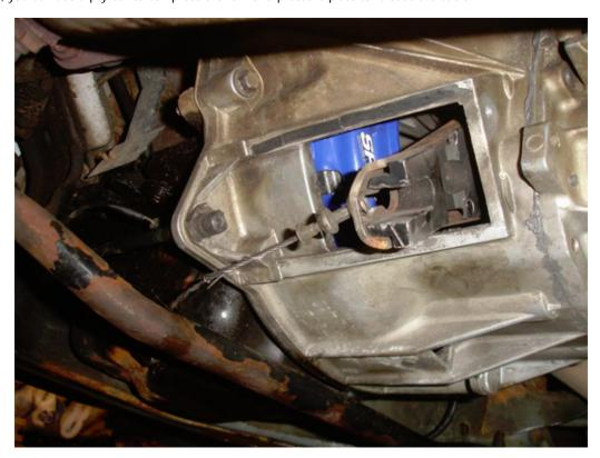
4. Then you will need to release the clip holding the cable to the transmission's bellhousing. You can use a screwdriver to pry it loose.
