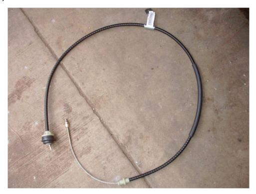
13. First thing is to run the cable from the top of the motor down to the bottom. The adjustable end will go down to the clutch fork and the non adjustable end will go inside the cabin. Run the bottom end between the k-member and the oil pan and then up to the firewall. Keep an eye on where the hanger is so that it fits up where it belongs on the side of the strut tower.
