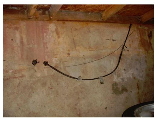
12. When you receive your new cable inspect it for any major defects or stuff like that. You will also notice the Steeda Adjustable Cable only has one hanger, this will be fine as it just needs to hold a bend and keep the cable away from moving objects such as the belt.
