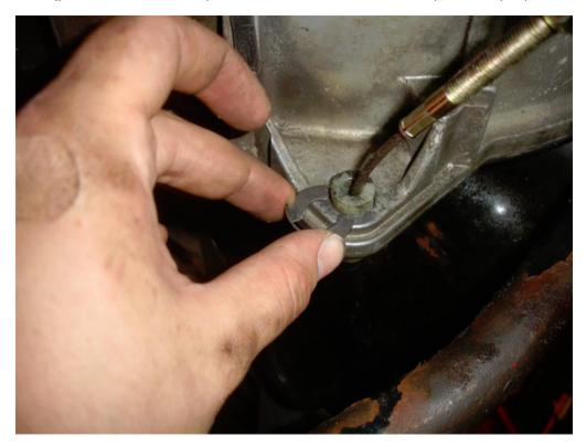
17. After the cable is now in place, go and put the bolt in the hanger for the cable. You can do this step earlier but I wanted to make sure everything had enough length and went into place before securing it.
