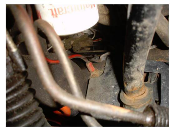
8. The last bolt is located up top by the oil filler cap, and below the brakes master cylinder. (Note: This was performed on a 96 GT and I noticed on my 98 GT that this bolt does not exist, so it may be there or it may not be.)
