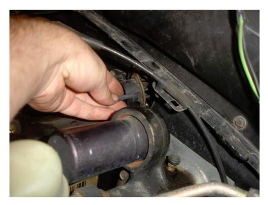
10. Your next step is to disconnect the cable from the clutch quadrant inside the car. You can find the quadrant above the gas pedal, the stock color is white. The cable should just slide off of the quadrant and then you should be able to pull it through the firewall (bulkhead).
