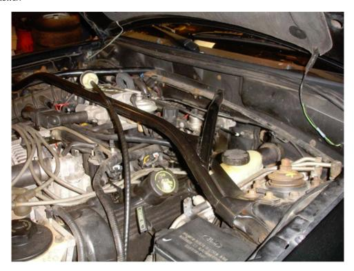
14. Next you will secure the rubber bushing/plug that fits into the firewall (bulkhead) where the stock unit was. The Steeda cable only uses one bolt to hold it in, so you can put the extra one aside.
