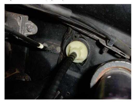
15. Now, inside the car you can run the cable into the clutch quadrant and slide it into place.
