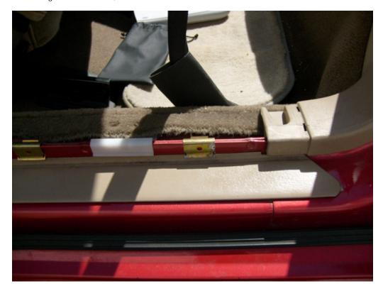
6. You will notice that the gold and white clips that I mentioned earlier might be touching the stock door sill. These clips might need to be lifted slightly so that you can remove the stock door sill. Use the flathead screwdriver or other prying tool to lift these clips.
