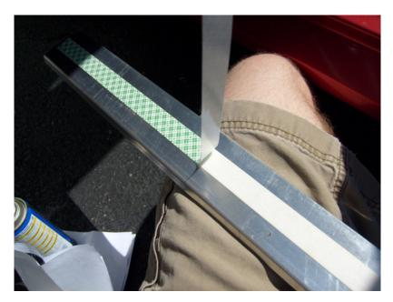
12. Once the tape is removed, place the door sill on the car. It should be centered between where the door trim was removed. There are also two lips in the frame where the door sill should center between.
