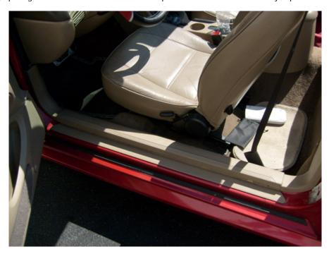
2. To start installing the door sill plates, the door sill trim cover needs to be removed.
