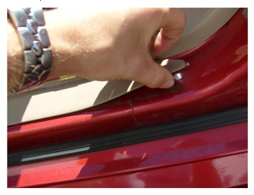
7. Besides the gold and white clips, the door sill is only held on with adhesive glue. To remove them, simply grab a corner and start to pull slowly, the stock door sill is pliable so don't worry if it bends. This is the piece that you will discard so don't worry if it is damaged in the process.
