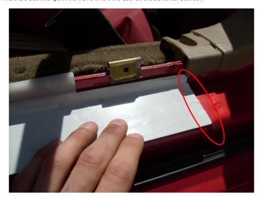
13. Once the door sill is in place, push down hard on the plate. Make sure the tape on the door sill plate adheres to the frame of the car.
