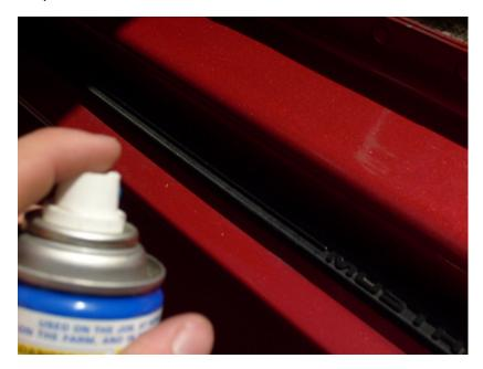
**Note:** Make sure the door sill surface is clear of all dirt, glue, and other debris so that the new door sill will adhere properly.
