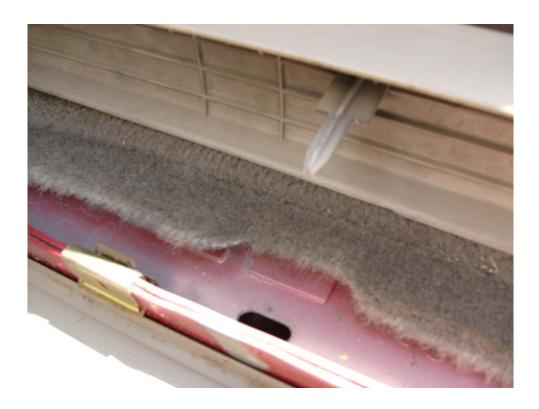
**Note:** The gold clips that are underneath the trim are designed to hold the two pieces of the frame together. The white clips are designed to hold the carpet down. Check all of the clips because some of my carpet clips where not it place.
