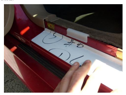
**Note:** It is important that the door sill is where you want it the first time. Trying to pull up the plate and move it around is very hard and the tape on the door sill may not stick as well as it could.
