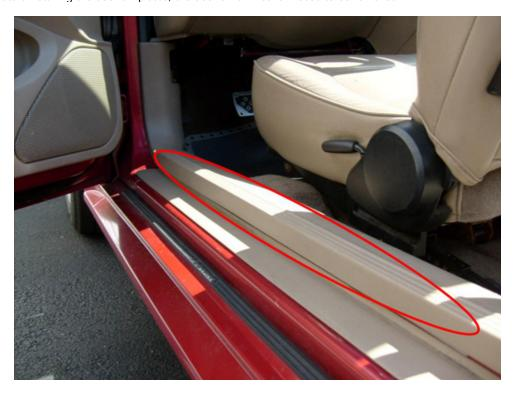
3. Start to remove the door sill trim by simply pulling up on one end of the trim. It is held in place by plastic pins that pop out to allow for removal. Do this slowly but with constant force and the trim will just lift out.
