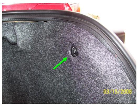
6. Using the door panel remover pry off the four retaining clips around the lock area.
