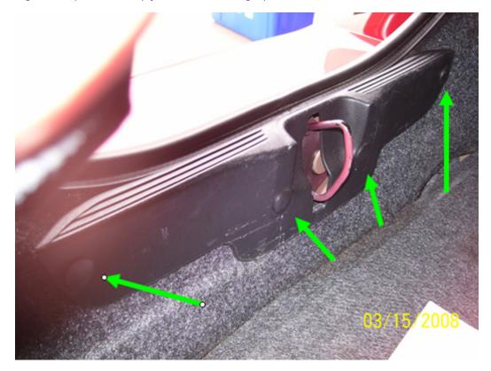
7. Remove the top plastic fasteners on top of the trunk by the hydraulic lift on both left and right sides.
