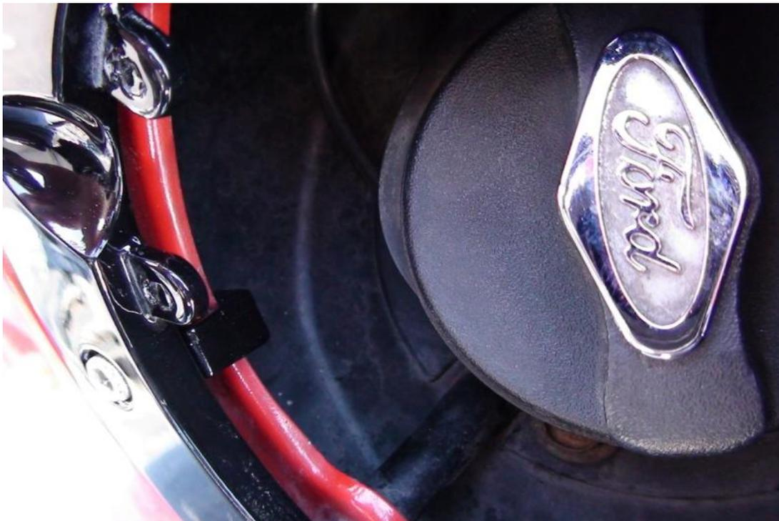
Once the hooks are in place, rotating the new fuel door while the rim is attached will not scratch the car. This is the best method for lining up the holes for the bolts rather than trying to line up the holes nearest the hinge of the door and attaching the hooks at the same time.
