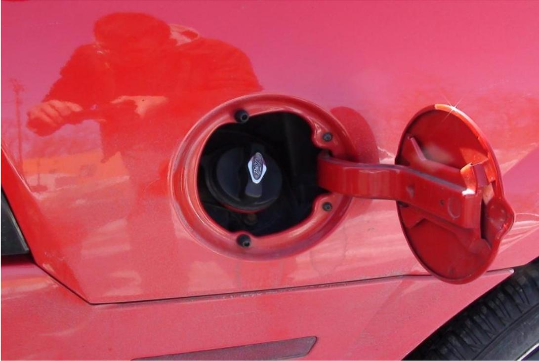
When removing the two screws holding the stock door on, make sure to hold the fuel door as you remove the second screw to prevent the door from swinging and scratching the car. Also, remove the gas cap or there will not be enough room for the stock fuel door to be removed.
