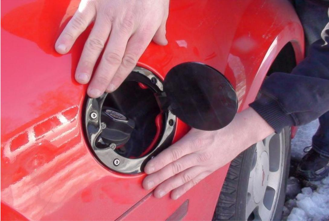
On the new fuel door, the holes for the bolts will line up with the holes in which the original stock fuel door attached itself too. Once lined up, insert the bolts and use the washers to attach the new fuel door to the car.
