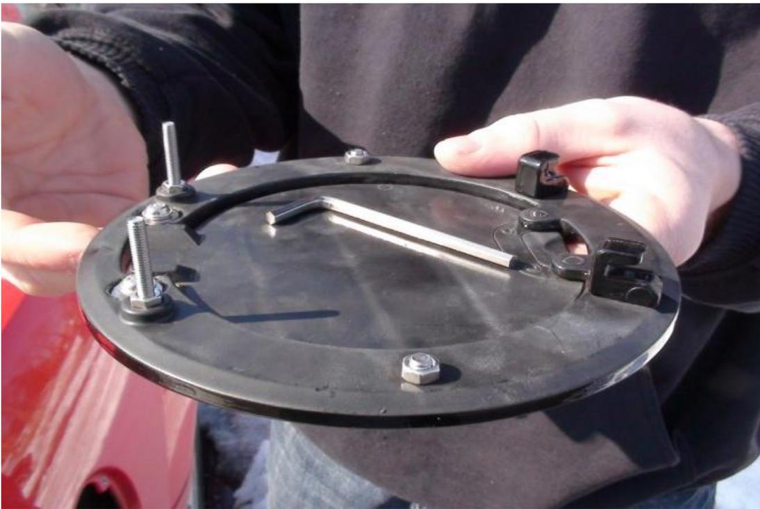
To the left, you can see there are a few nuts on the back of the fuel door. In order to properly attach the door, you must remove all of the nuts from the bolts. When clear, you are ready to begin attaching the fuel door to the car.
