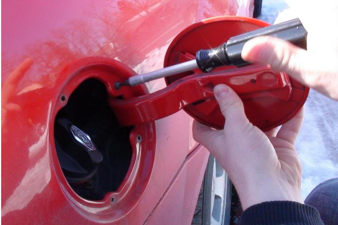
As you can see, the hinge the stock fuel door is connected too is very large and can be difficult removing with the gas cap still attached.
