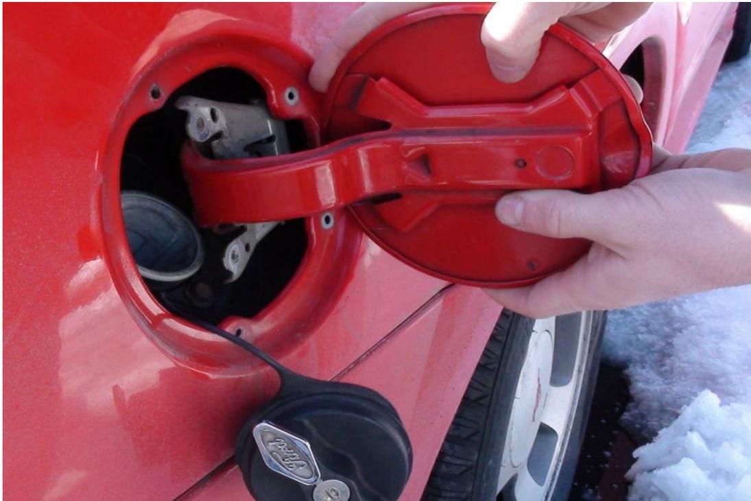
**Stage 2: Preparing the new fuel door for installation.**
