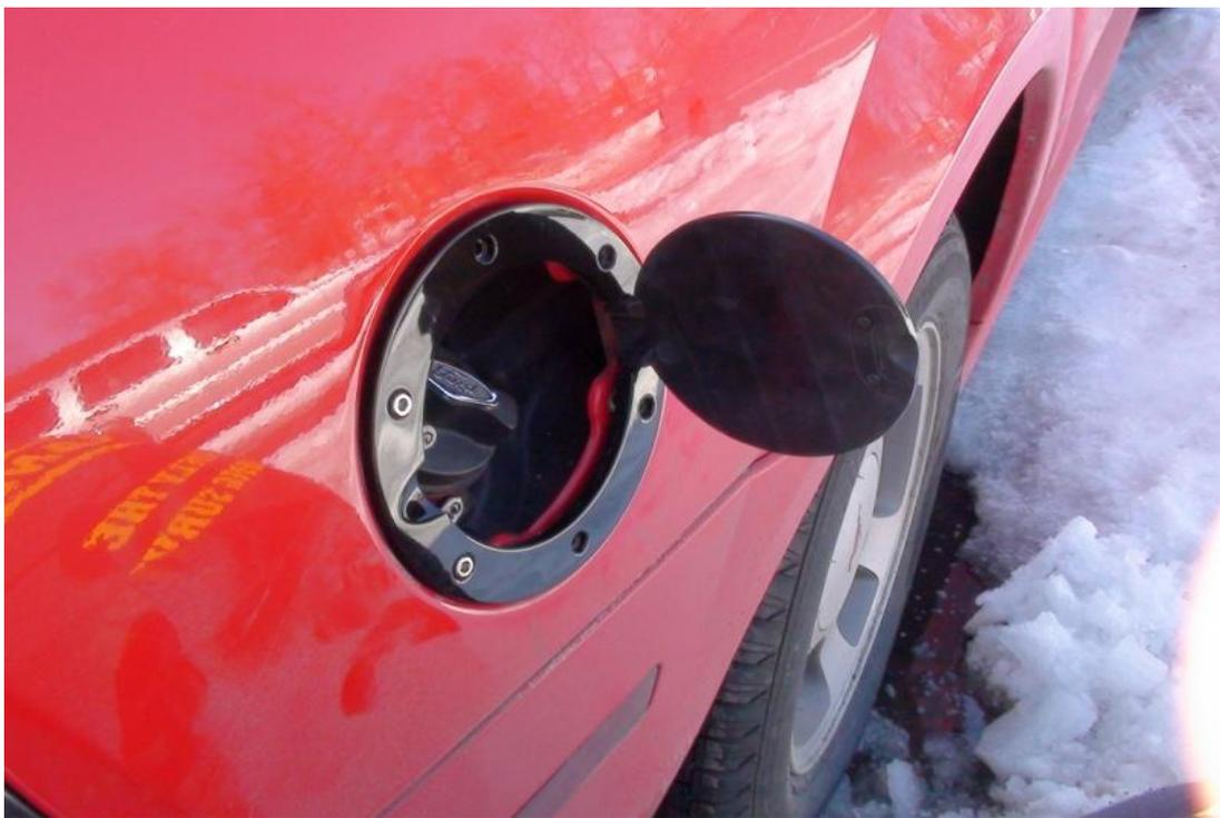
Use a socket wrench inside the fuel door compartment to hold the nut in place as you use an Allen wrench to tighten the bolts that hold the fuel door in place. As this part is the trickiest part of the installation, take great care when using the Allen wrench so you do not scratch the outside of your new [fuel door](#). Be sure to tighten the fuel door as best as you can to make it lay flush with the rest of the car.
