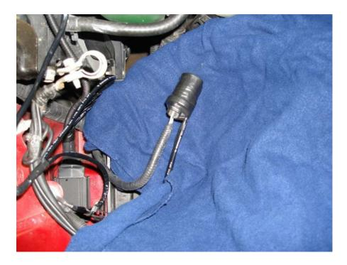
7. We mounted the driver side ballast on the side, behind the battery using double sided tape. Since the ballast is thin, it will not interfere with the battery and once the battery is back in place it cannot be seen. Connect the ballast to the main harness and bring over the 3 wires for the new lamp through the hole. Neatly tuck and zip tie all the wires out of the way of moving parts.
