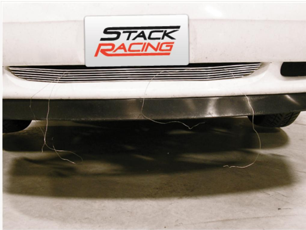
5. Twist the wires until the grille is held securely in place. Trim excess wire with wire cutters and wrap the ends of the wires in electrical tape to prevent scratching your paint.
