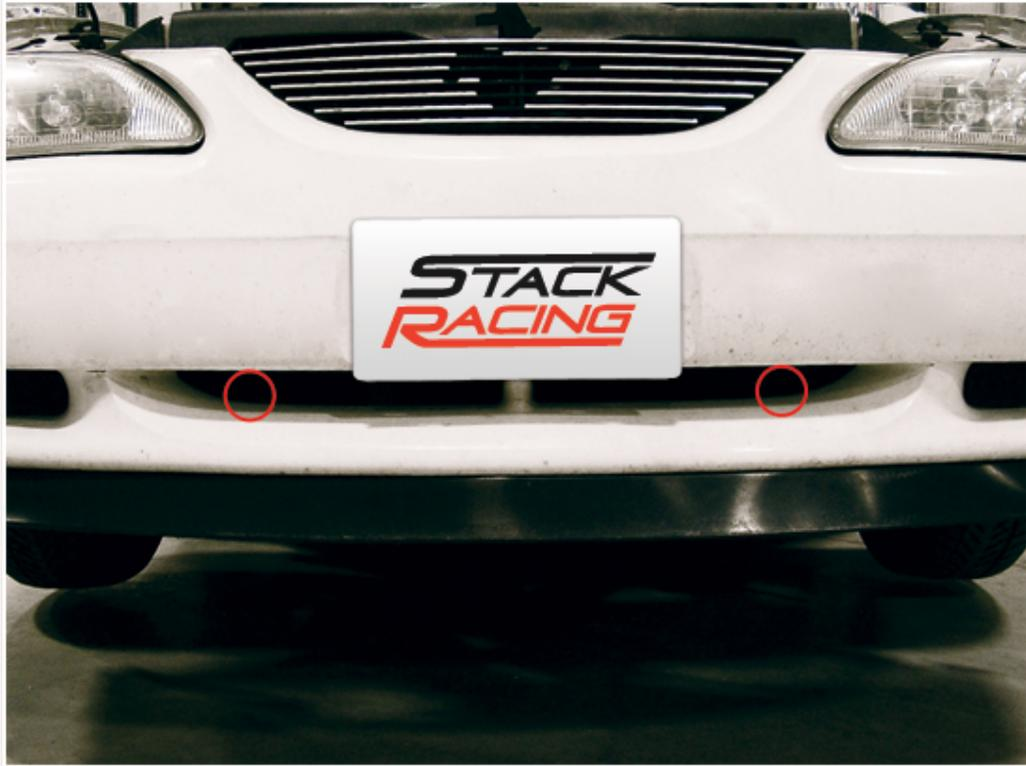
4. Center your grille. Have your assistant hold the grille in place. From the back of the grille, thread the two provided wires through the clips and then back through the front of the grille, wrapping them around the side bars of the grille.
