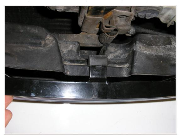
4. Using a 3/16" bit, drill a pilot hole in each of the locations you marked above.
