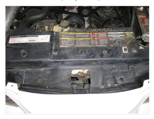
2. To remove the pony and its bracket, simply unscrew the 2 Phillips head screws that are holding it to the vehicle.
