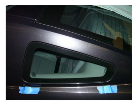
4. Then measure 1 inch from the edge of the window on top and bottom and place a piece of tape along the edge so it is even. I found that the 1 inch from the edge followed the roof line best.
