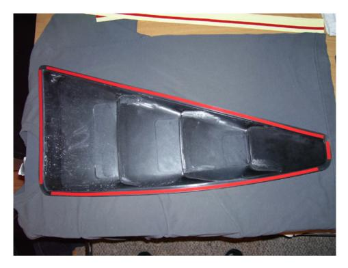
7. Peel off the leading edge of the protective coating to get ready to place it in position.
