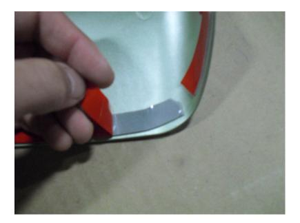
3. Lightly place the mirror cover over the mirror, taking care to align the cover in the corners properly.
