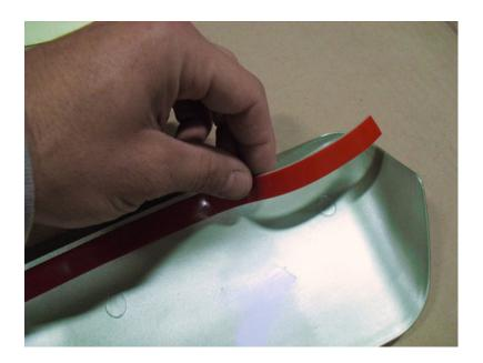
2. Peel the backing from the adhesive tape on the mirror cover.
