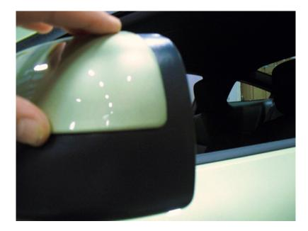
4. Once the mirror cover is in the desired location, firmly press down on all the surfaces where the adhesive was applied, to ensure a proper fit.
