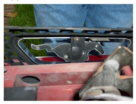
6. Once the fasteners are off, simply pull the stock pony off the front of the grille.
