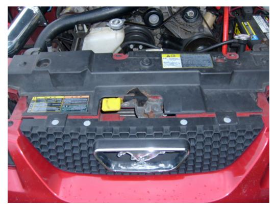
3. Taking a set of pliers and a screw driver, remove each pushpin. Try not to damage the pushpin during removal because they will be needed to install the grill back into place.
