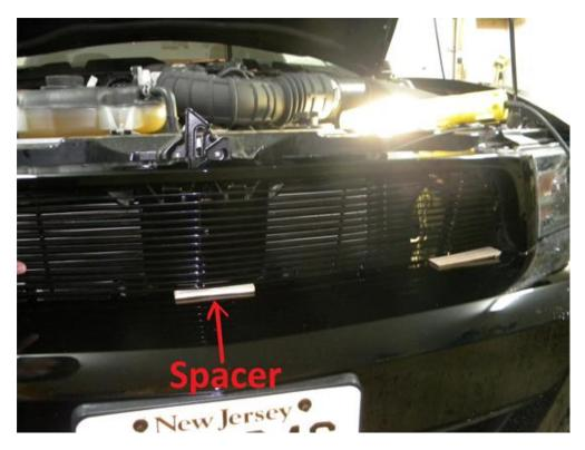
5. Locate the mounting tabs on your new grill and pre drill the hole. After your hole is predrilled begin to set the screw in but don't let it go too far. The locking clips should be set on the screw, as its peeking through the other side of the plastic and then the screw should be drilled in the rest of the way. This will allow for the locking clip to bind onto the plastic and hold the grille in place. Do this for all three mounting tabs.
