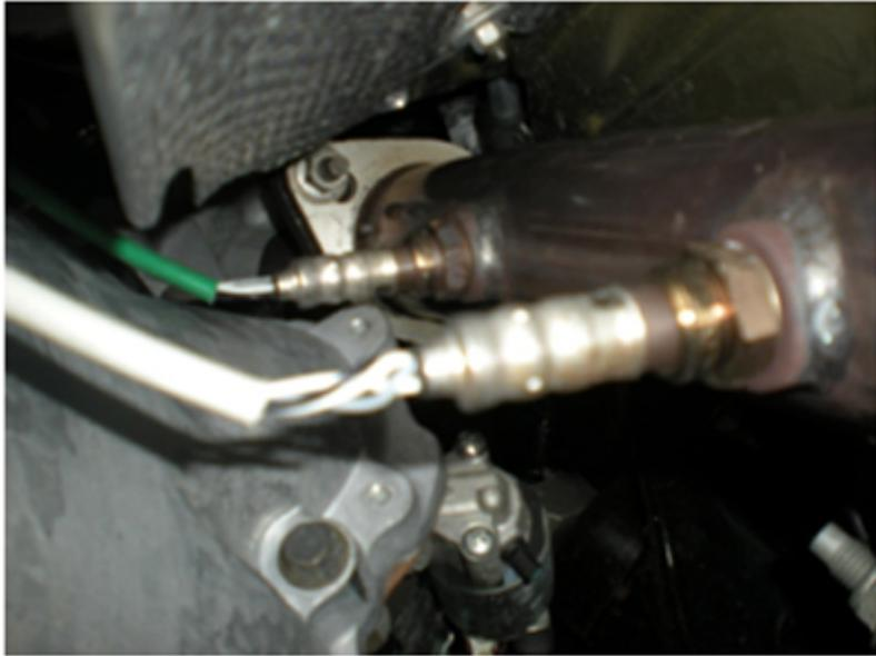
6. Now use the channel locks to unscrew the 3 O2 Sensors from your stock H-pipe, there should be 2 on the passenger side and one on the driver side. Once unscrewed and removed you can just let them hang until re-installation.
