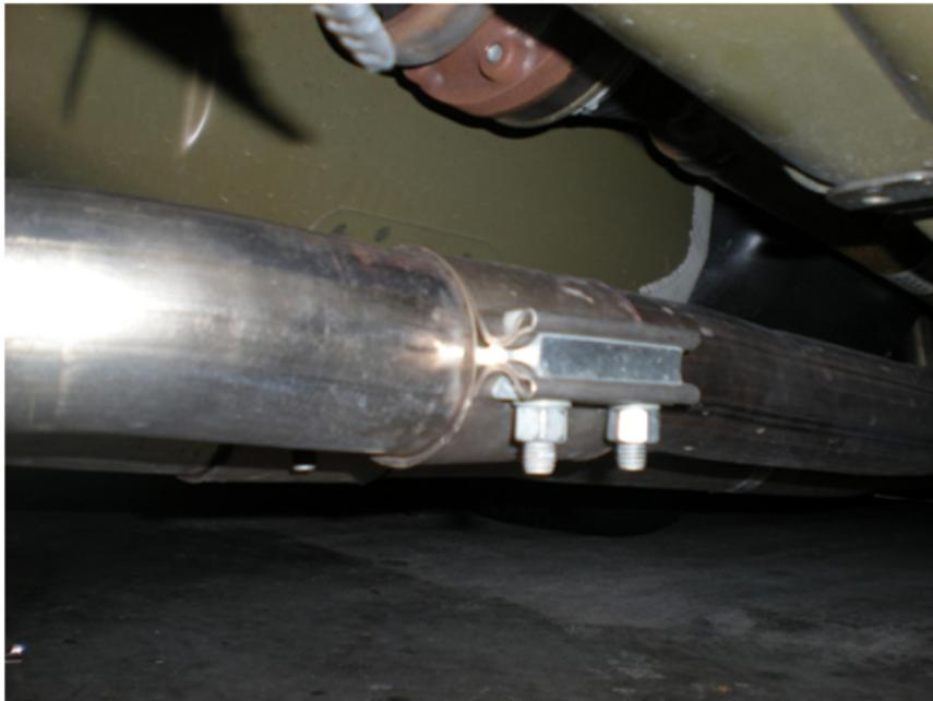
8. Next, slide the ring clamps that connect the down pipes to the mid pipe over the connections. Make sure to get the as close to the front of the connection as possible to prevent exhaust leak. Now tighten these nuts down, keeping the clamp behind the bolt, over one of the slits in the pipe to prevent leakage. Tighten as hard as possible.
