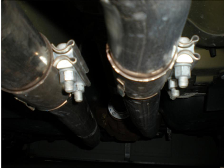
3. Find where the stock H-pipe connects to the rear pipes that go to the mufflers. There should be two sleeves, one on each pipe that connects the mid pipe to the rear pipe.
