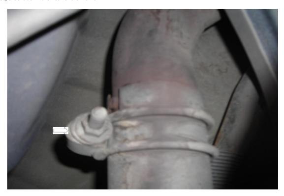
2. Remove exhaust clamps by loosening the bolt holding it in place with a 15 mm wrench and sliding it down the neck of the muffle
