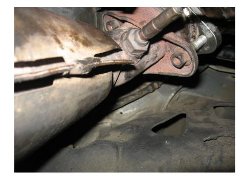
7. Using the 5/8" Socket, unbolt the 4 bolts attaching the exhaust manifolds to the mid-pipe (2 on each side). The bolts are attached to the stock exhaust manifold, unless you've upgraded to aftermarket headers.
