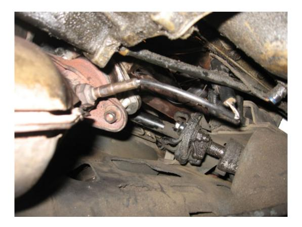
4. Unplug the O2 sensors by pushing in the small tab and pulling to disconnect them.
