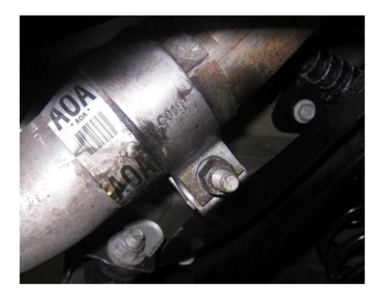
4. Use a ratchet and 13mm socket to remove the bolts holding the hanger closest to the tire. You will need to use a 13mm wrench to remove the bolt above the muffler because there is not enough room to fit the ratchet and socket. (Repeat for opposite side).
