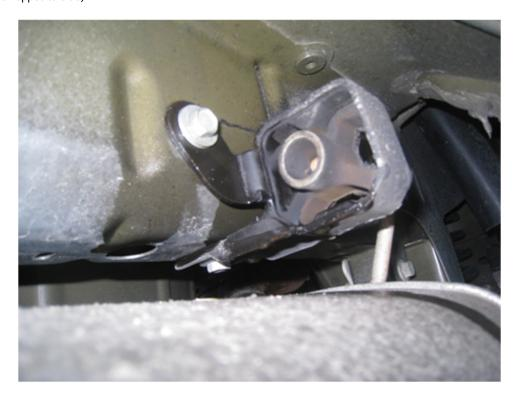
5. Use a ratchet and 13mm socket to remove the bolts holding the hanger closest to the bumper. Use the 6" extension for bolt (2) for easier removal. This will allow you to clear all components of the car and have more freedom of movement. Once all the bolts have been removed, you can remove the axle-back exhaust. You may have to wiggle and turn the exhaust back and forth to get it off of the mid-pipe. (Repeat for opposite side).
