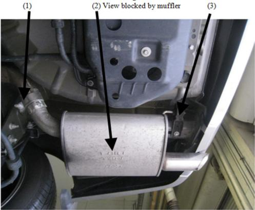
3. Use a ratchet and 15mm socket attachment to loosen the bolt holding the factory installed pipe clamps. Once the clamp is loosened, slide the clamp down the muffler neck. Due to road grime and rust, it may take some break-free spray or a few light taps with a hammer to loosen the clamp so you can slide it down. (Repeat for opposite side).
