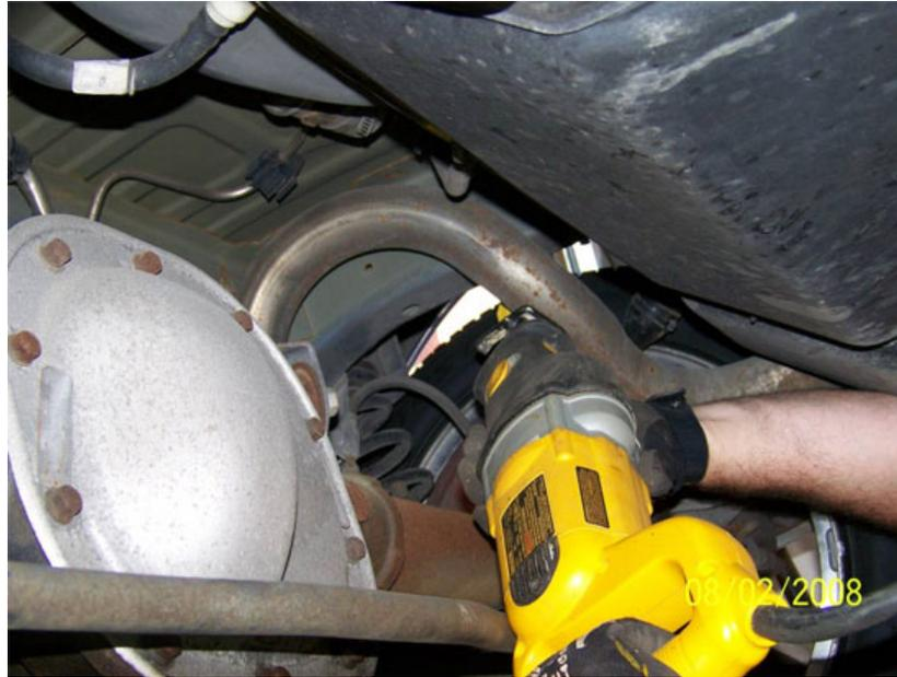
11. With the factory exhaust removed now you can work the new, over-axle portions into place. This part can be a bit tricky. Be patient and do not attempt to do this without first taking BOTH rear wheels off. The long section faces the rear while the hanger faces the cats. Remove the black packing material from the Pypes hangers and slide them into the factory grommets (additional WD-40 may help).
