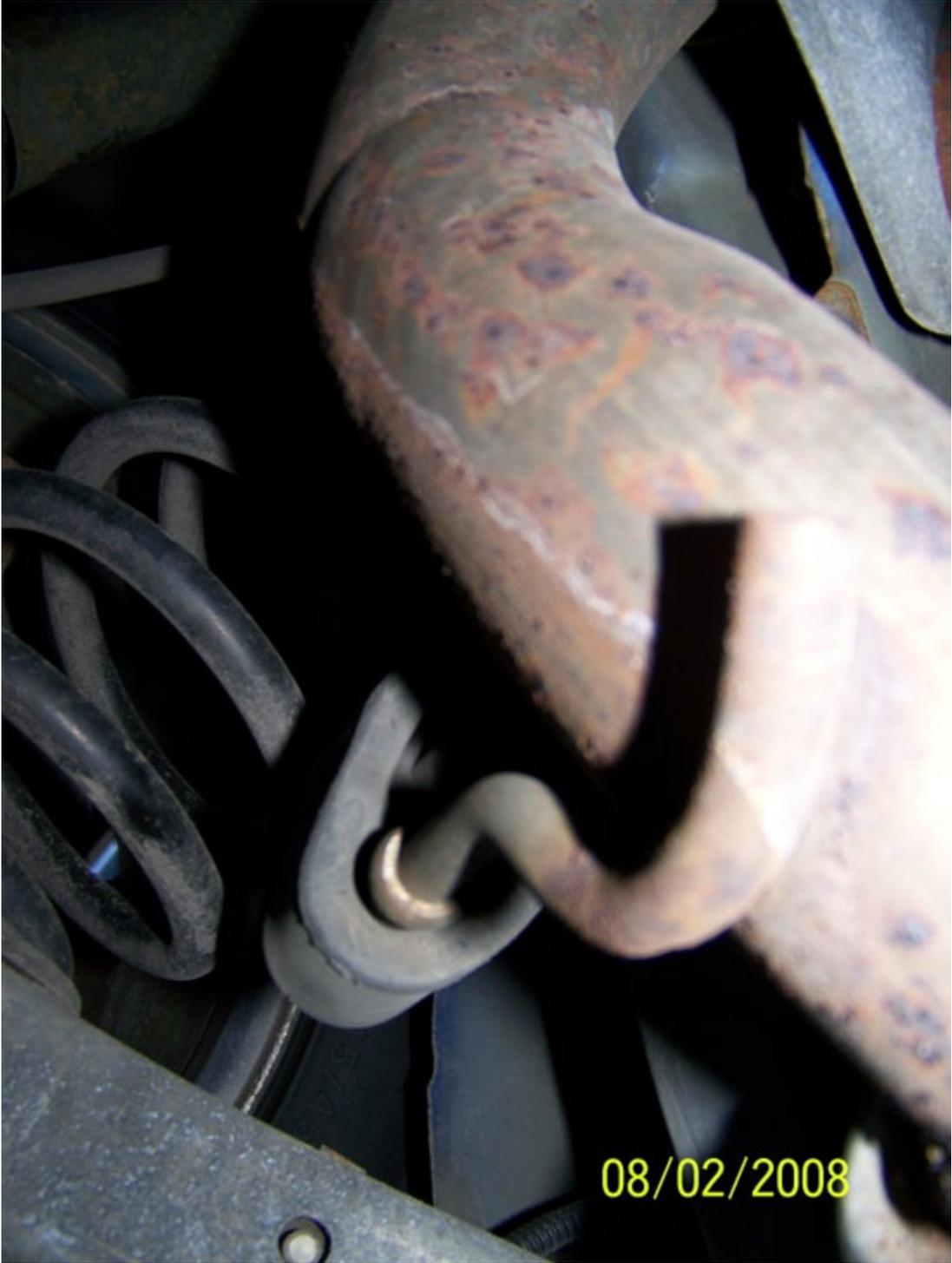
9. Break the 14mm nuts free, which hold the factory exhaust on. Since we used the "PB-Blaster" beforehand, we were able to easily break free the nuts with hand tools. The studs are firmly attached to the H-pipe flange and do not require a second ratchet or wrench to hold.
