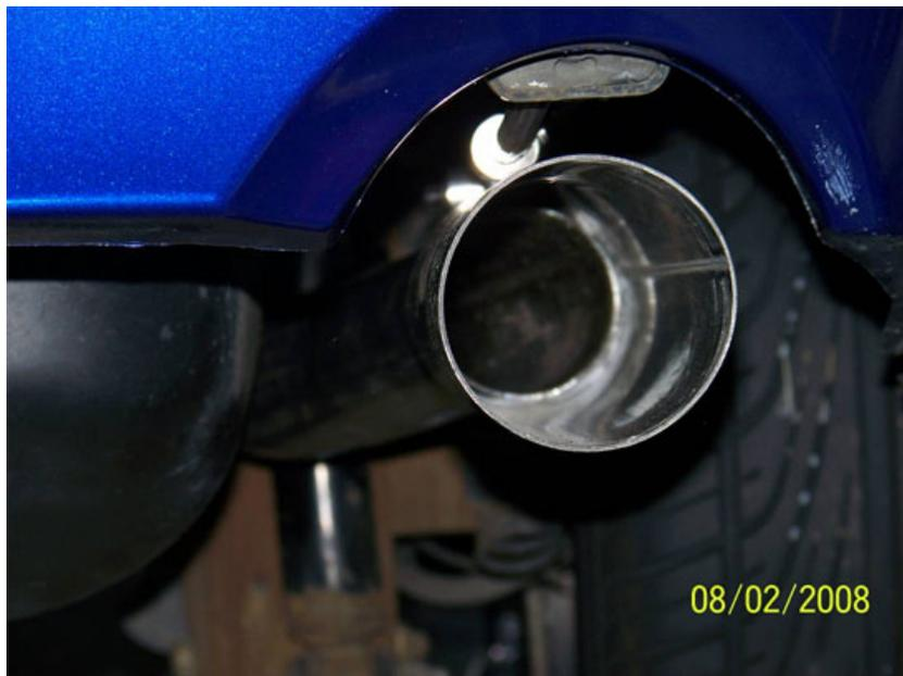
13. Slide another clamp onto the flow tube and slide it into the muffler. The flanges are floating and allow for proper fitting to the H-pipe. If you go in any other order you will be frustrated by parts not having clearance to fit.
