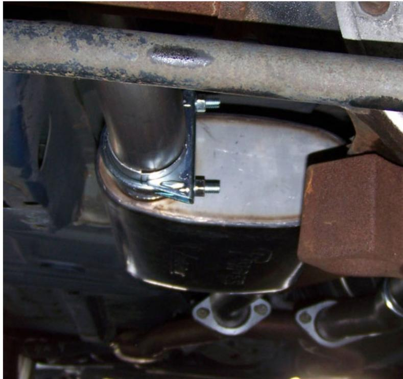
18. Once everything is loosely in place go ahead and tighten all connections. Have a friend hold the exhaust system up while you tighten it down. Make it TIGHT. Work on each nut a few turns at a time then switch to the other. Attempt to leave equal threads visible on each side of the U-Clamp.
