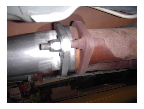
4. The catback hangs at two places; one is right behind the muffler and another at the tailpipe. The pipes are hung by a rubber hanger. These can be a little tricky to remove, but a spray of WD-40 the night before can help in removal. Pry the metal hanger out of the rubber hanger with a flathead screwdriver. Remove the metal hangers from all four rubber hangings. If your rubber hangers are in bad shape, it would be a good time to replace them now.
