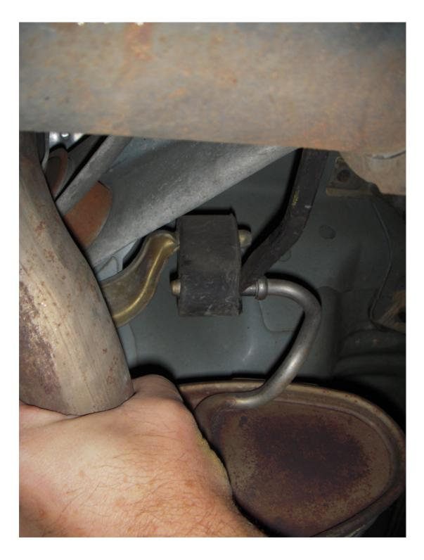
5. Now it is time to remove the system. But seeing it is one long pipe you will need to cut it with a hack saw to remove it. You will need to cut the old pipes somewhere on the arch where it goes over the rear axle. Once you saw through it and have two pieces, pull them over the axle to get the old pipe out of the way. Do this for both sides. See image for hacksaw positioning.
