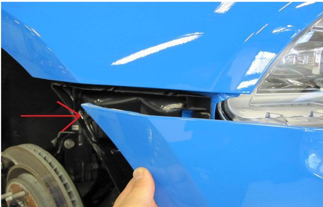
7. Now you will have access to the two lower bolts holding the headlight assembly in place. Using a 10mm socket, remove the two lower bolts and one upper bolts on each side and remove the factory headlight assemblies.
