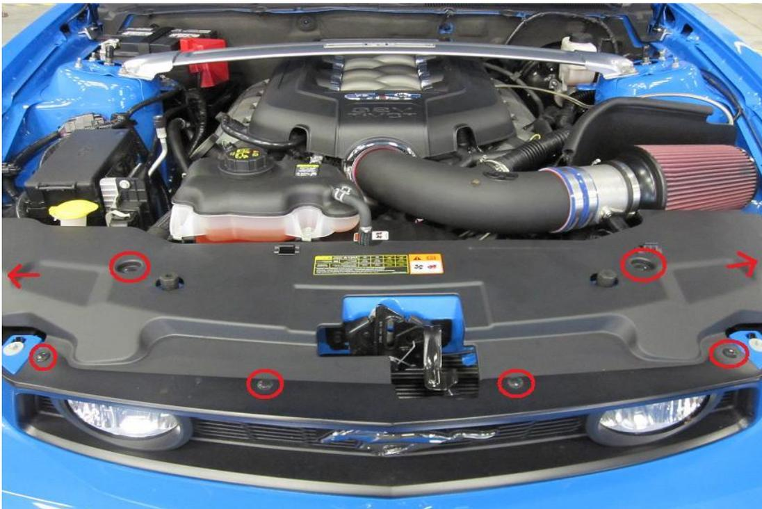
5. Remove the two 8mm bolts holding the top of the front bumper cover on and pull the cover over the black plastic tab shown in the photo below.
