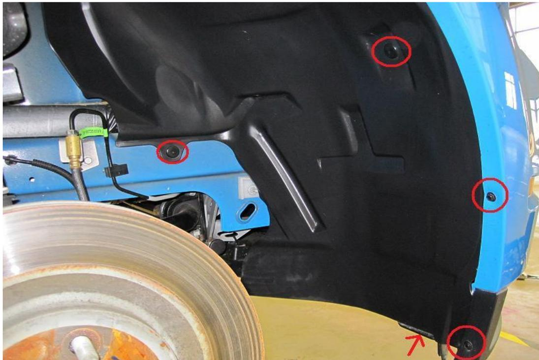
3. Remove the four 7mm sheet metal bolts holding the splash shield to the underside of the front bumper cover.
