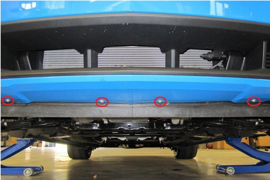
4. Remove the eight plastic retaining clips holding the plastic radiator cover on. Then remove the cover from the vehicle.
