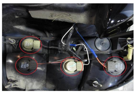
4. Install the bulbs in the new housing in the same position as they were removed from the old housing.
