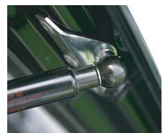
Rotate clip until it snaps onto shaft.
