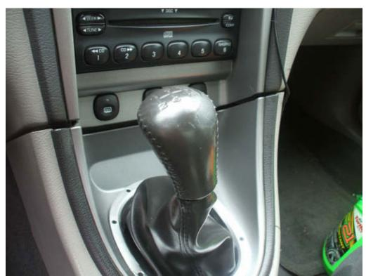
1. Removing the stock shifting knob is easy. All you have to do is grasp the knob with your hand and twist it counter clockwise. The knobs are merely screwed onto the shifter.
