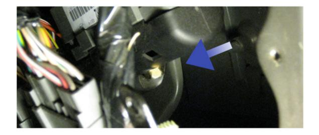
6. Once the bolts are removed, slide the computer out. The plastic covering of the J3 port needs to be removed. Take a screw driver or pliers, whatever you have around, and on the opposite side of the where the computer was connected, gently slide this item under the tab to remove it.
