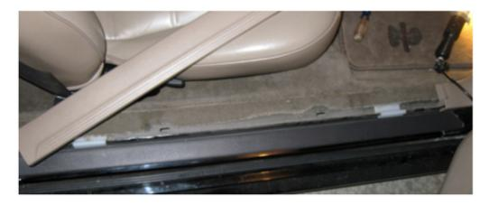
3. To remove the kick panel, just put your hand behind it and pull straight out on the tab. It comes right off.
