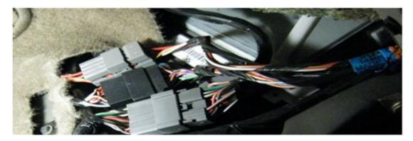
5. Next, you will have to take the 7mm Socket and remove the two bolts holding the bracket attached to the three connectors. After the bracket is free, you can now get your hands in towards the computer. Unscrew the one 10mm bolt on the bottom center of the computer and the one small golden 5.5mm bolt holding the plastic box that secures the computer.
