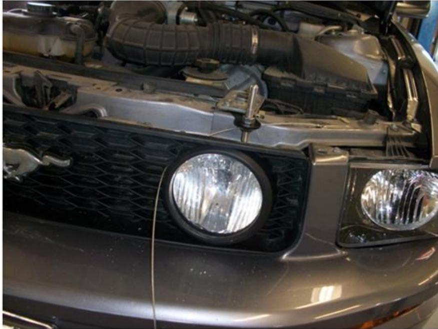
16. Cut holes in the radiator cover and reinstall in reverse of removal.
