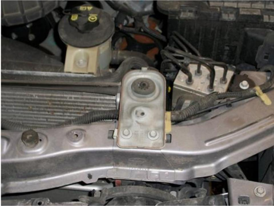
4. Install metal brackets underneath radiator support. Brackets must face towards outside of engine compartment, as shown here from the driver's side. Tighten bolts.
