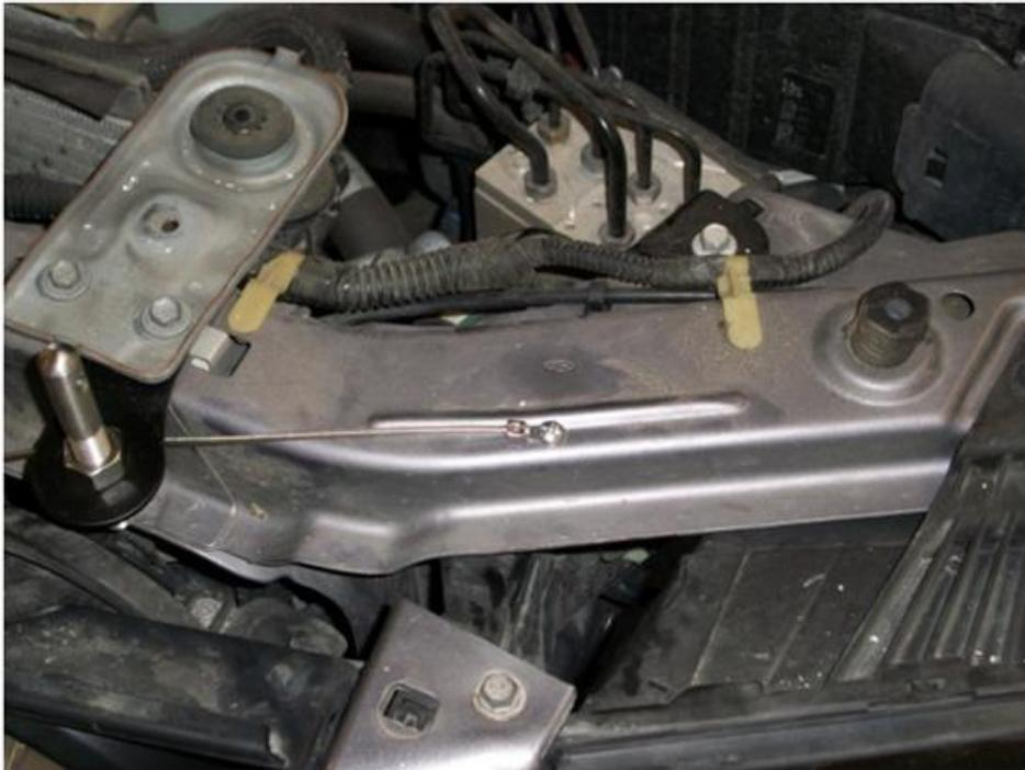
15. Route lanyard around brackets and place through corners of the grille. (Fig 8)
