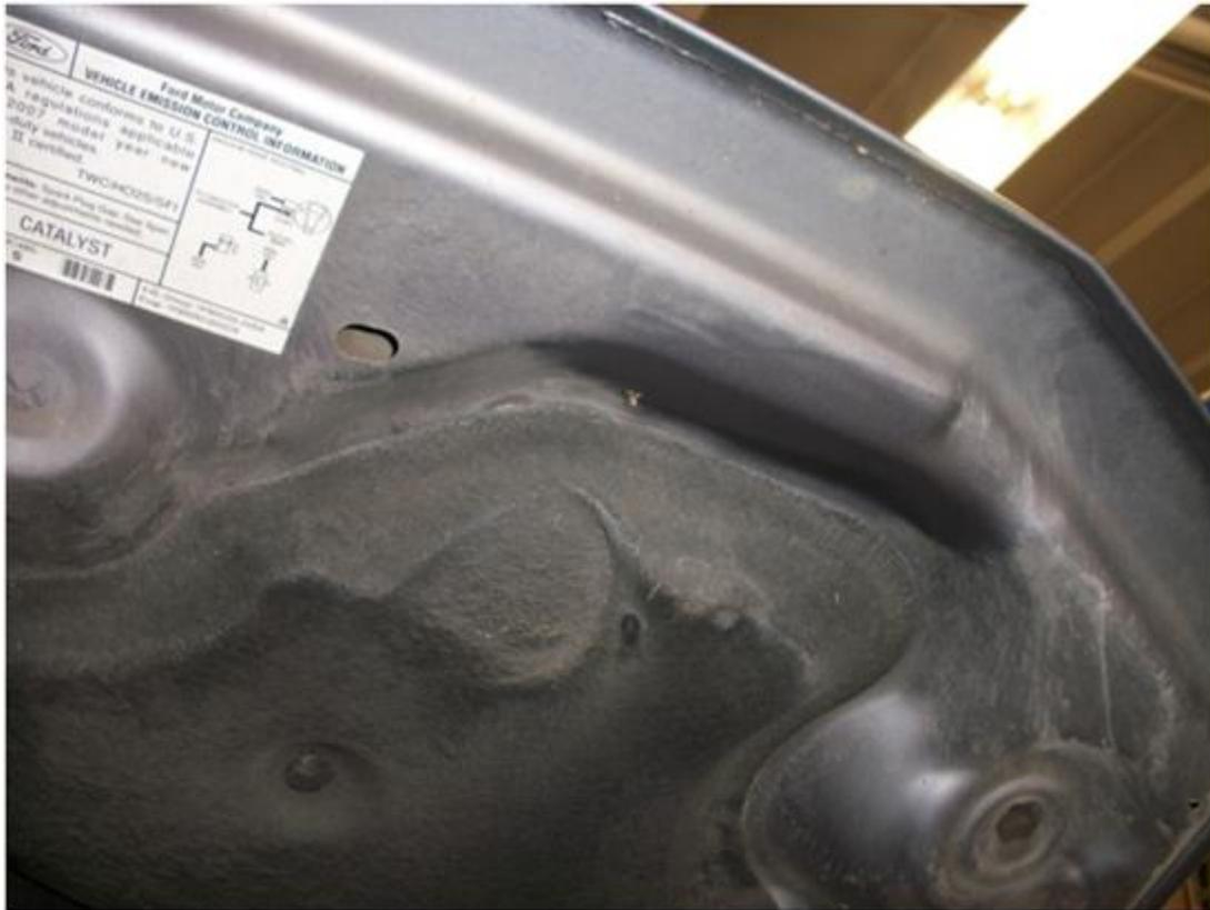
7. Using 1/8" bit, drill a starter hole directly through the hood on both sides. Keep in mind that the hood will be slightly angled compared to the hood pin, so drill bit must be angled as well to make hole as straight as possible.
