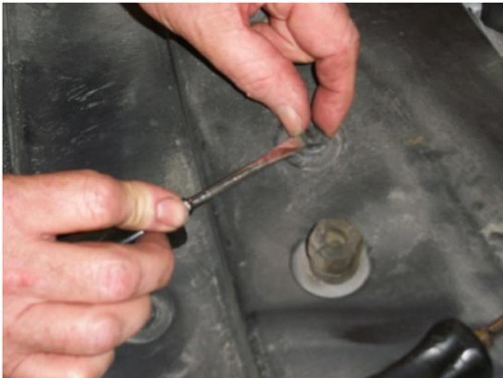
3. Loosen and remove both radiator support bolts on either side of the radiator.
