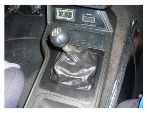
3. With one hand hold the shift knob tightly and with your other hand hold the shifter neck under the shift knob tight so that you can break the shift knob loose. Start by twisting the shift knob to the left (counter clockwise)so that it will loosen. Keep turning until it completely comes off.
