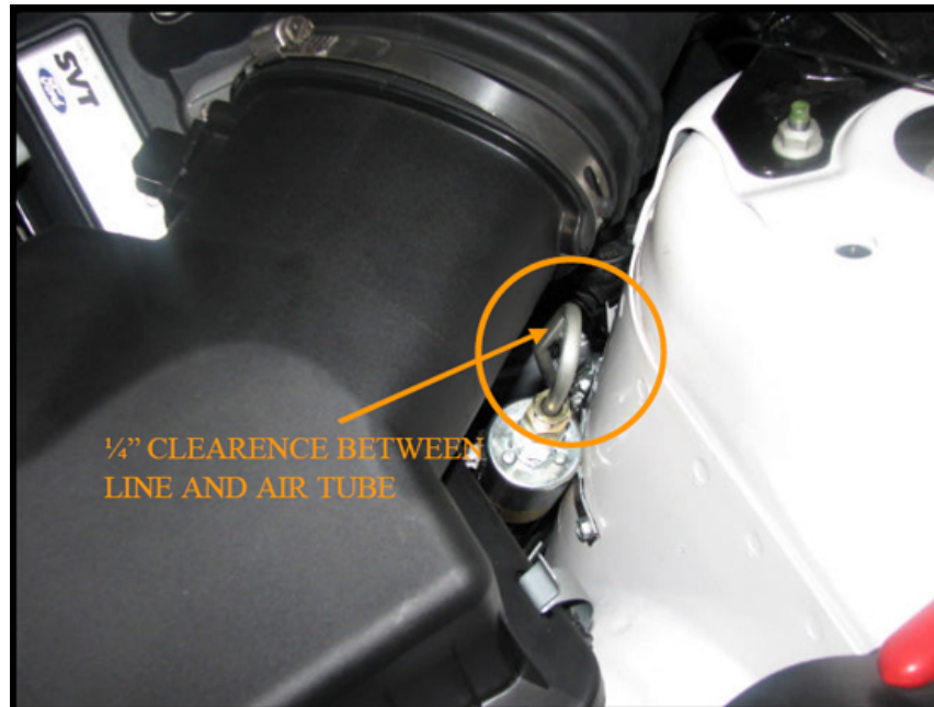
Line Lock Final Install Position
