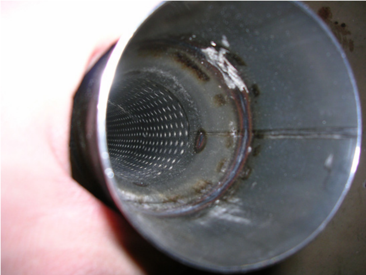
Inside the Loudmouth II Bullet Muffler
