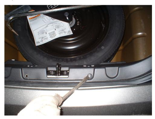
3. Remove the 3 nuts from the tail-light assembly studs. Pull the carpet back behind the tail-light to gain access to the mounting hardware. Remove the 3 nuts with an 11mm or 7/16" wrench.
