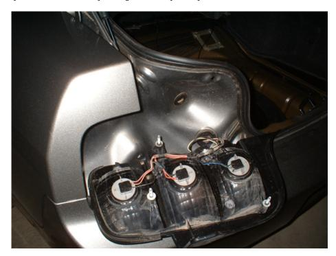
6. The wiring fastener must also be removed from the old lights by pulling it out (see picture above); please note that as far as I can tell there is no place to re-attach this fastener on the new tail-lights. There is a drainage port in the place where the fastener went on the old tail lights. Do not try to force the fastener into this hole, as it will not fit.
