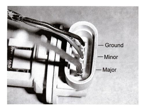
4. Install the gasket onto the wires and slide it back into the socket. If the lamp you removed is a dual filament lamp, then put the lamp back into the socket. Otherwise, obtain a #3157 lamp and install it into this socket.
