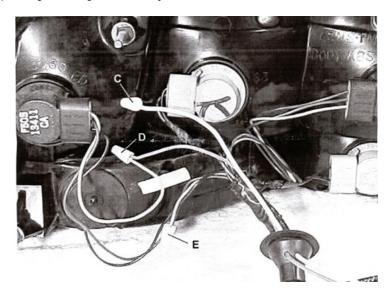
13. For the Left Side of the car, repeat the above steps using the other sequencer module. Note that the colors of the car wiring are different on this side of the car. The MAJOR wire on the Left Side is green with an orange stripe.
