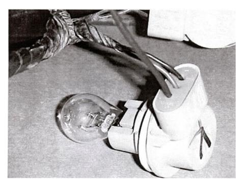
5. Remove the middle socket from the tail light fixture. Insert the inside socket into the middle position, and insert the middle socket into the inside position. There is room for this swap, but since each car is different, you might have to unwrap some of the harness tape, and/or pull a clip out of the car body.
