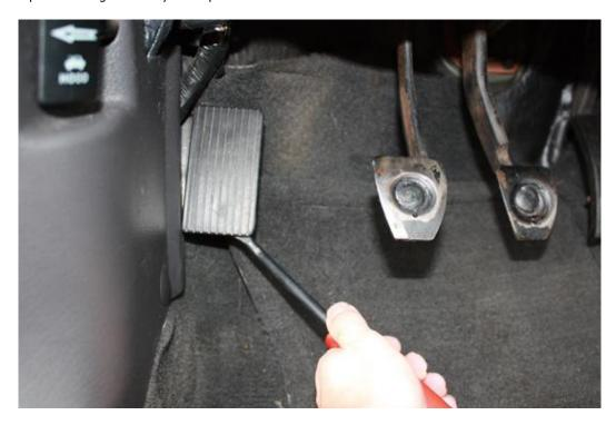
3. Remove the accelerator pedal. To remove the accelerator pedal you will need a socket or wrench. Once the two nuts are removed you will need to detatch the throttle cable from the top of the pedal. To do so, lift the pedal assembly up to give the cable slack and pull it down out of the grove.
