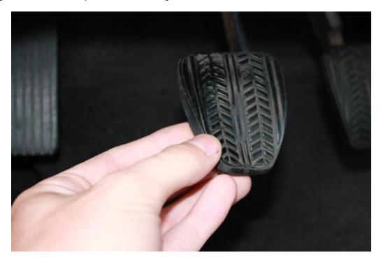
4. The installation of your new pedals. Start with the easiest first. The dead pedal. The dead pedal uses two clips to attach. Simply put into place and press. Use foot if needed.
