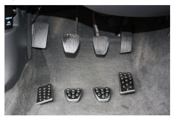
2. Remove the dead pedal. The removal of the dead pedal will require either a large flat head screwdriver or an interior trim removal tool as seen in the picture. Place either tool between the dead pedal and the metal bracket and pry it off. The pedal is being held on by two clips.
