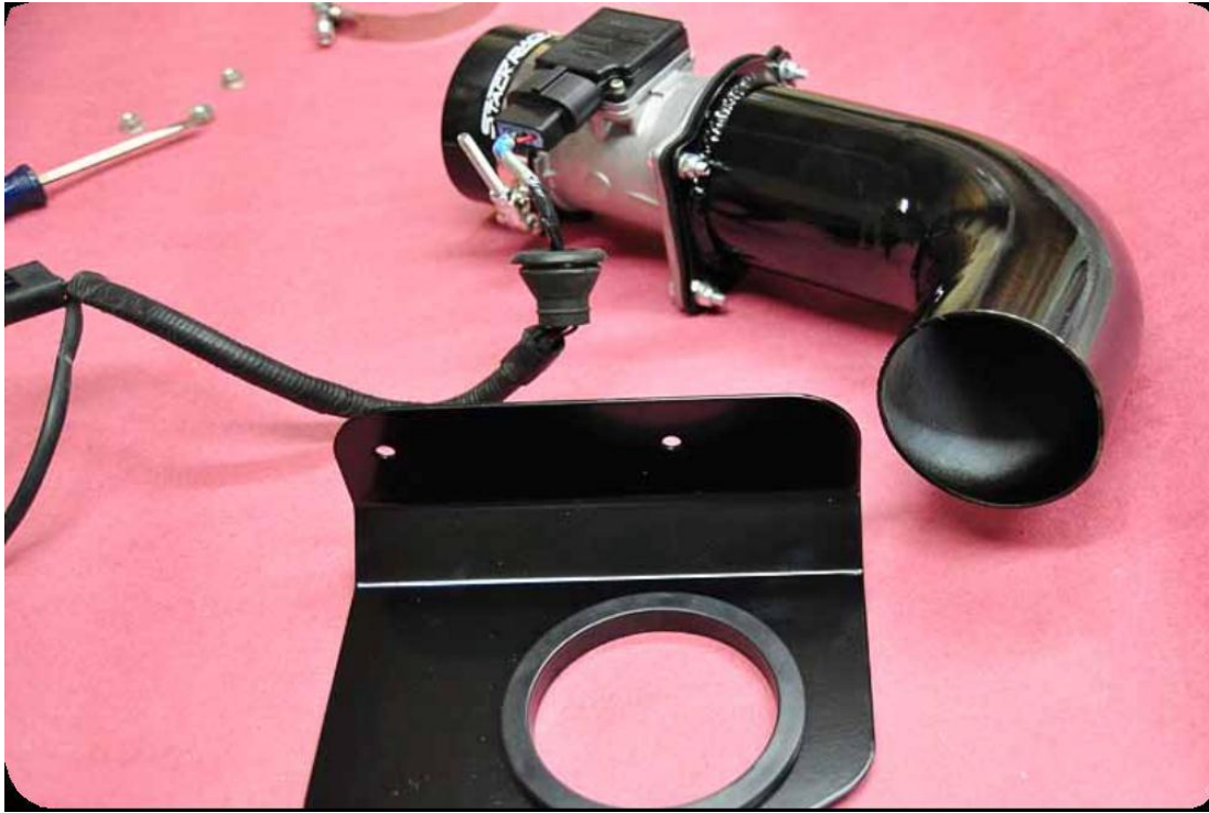
Rubber grommets that will accept the support bracket.
