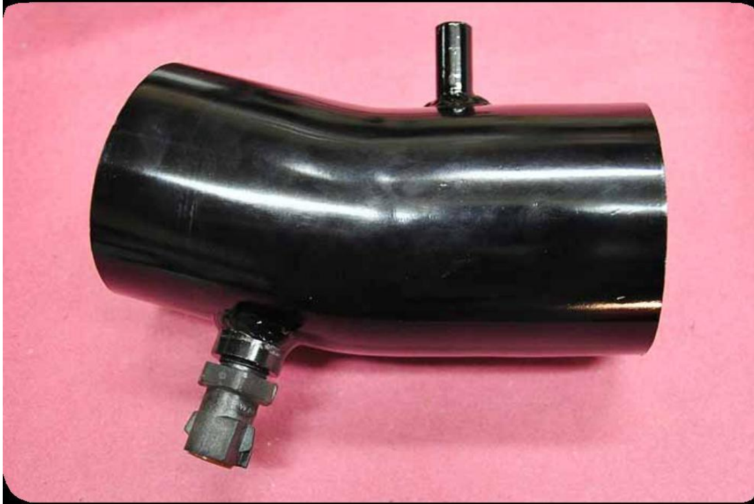
Intake tube with mass air flow sensor installed.
