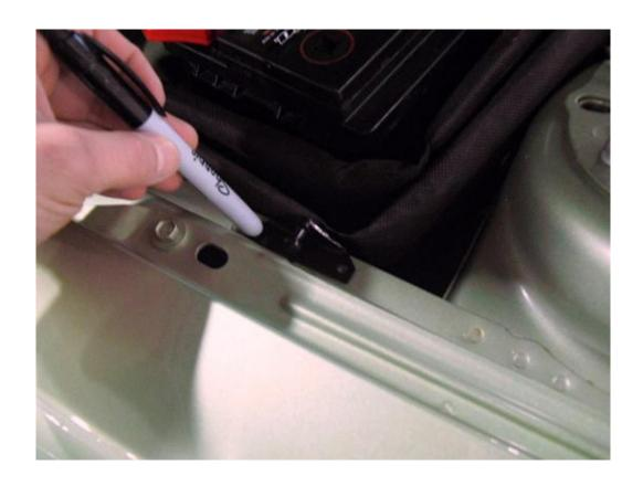
7. Drill two 5/32" holes where you marked on the inner fender.
