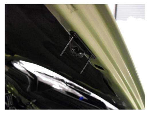
5. Slide the rivet gun over end of rivets and, using firm pressure, press the handle on the gun a few times until rivet gun pops and snaps off stem of rivet.
