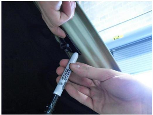
3. Using a power drill with a 3/16" bit, drill two holes on the underside of hood where you marked with the black marker.
