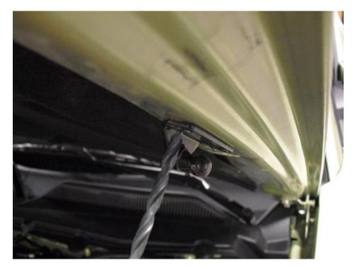
4. Place two rivets inside of the holes that you have just drilled. It will be a tight fit, so you may have to twist the rivet a bit to get it into the hole.
