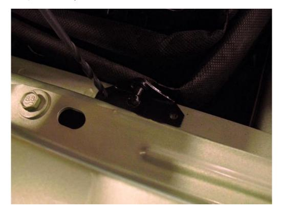
8. Use a ratchet and an 8mm socket to secure brackets to inner fender using supplied screws.
