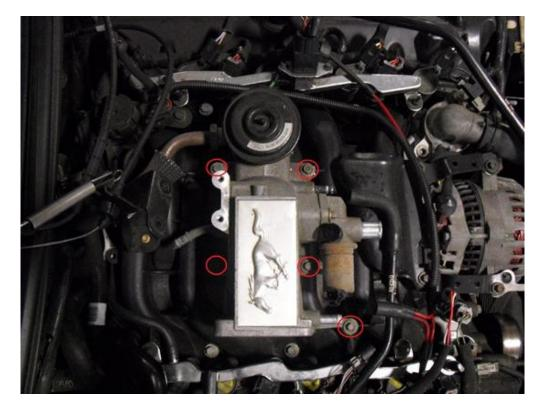
6. Once the factory plenum is removed from the vehicle, remove the two 8mm bolts holding the IAC valve on and remove it from the factory plenum.
