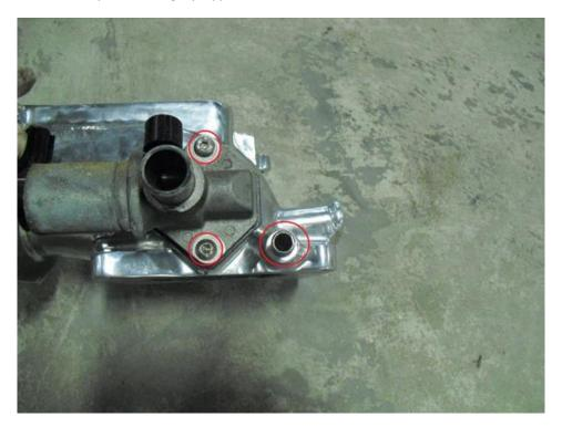
8. Install the Stack Racing plenum onto your factory intake manifold using the five 8mm bolts you previously removed.
