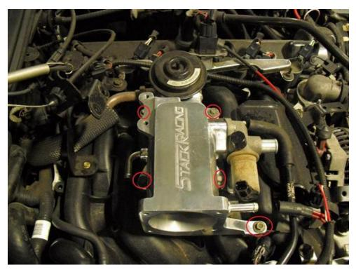
9. Re-install the vacuum hose on the rear of the plenum, along with the throttle cable bracket and throttle body using the bolts you previously removed.
