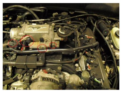
3. Remove the two 10mm bolts holding the throttle cable bracket in place, the four 8mm bolts holding the throttle body to the plenum, and the vacuum hose on the rear of the plenum. When throttle body is loose from plenum, carefully rest it on the vehicle's cowl panel so it is out of the way.
