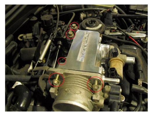
10. Re-install the two bolts for the EGR valve, and reconnect the TPS and IAC harnesses, as well as the PCV vacuum supply and vacuum block connections.
