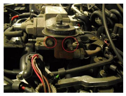
5. Remove the five 8mm bolts holding the plenum to the intake manifold and remove the plenum from the vehicle.
