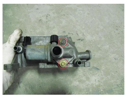
7. Install the factory IAC valve onto the Stack Racing plenum using the two supplied Allen head bolts. Make sure to use the new supplied gasket for the IAC valve. Also take this time to press in the PCV vacuum hose adapter into the plenum. There are two sizes included, so you will have to determine which one you will need depending on the size of your vacuum hose. The adapter can be lightly tapped in with a hammer.
