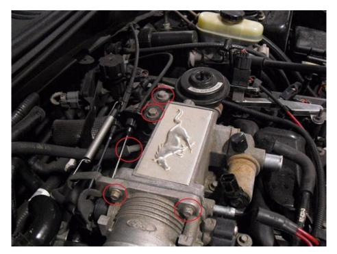
4. Remove the 10mm bolt and the 10mm stud holding the EGR valve to the plenum.
