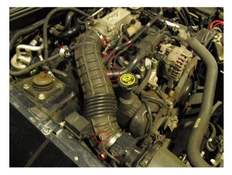
2. Disconnect IAC hose, PCV hose, and vacuum block from plenum. Also remove the TPS and IAC harnesses at this point.
