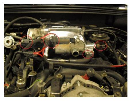
11. Re-install the air inlet duct, reconnect the air supply hoses on the intake duct, and reconnect the IAT harness.
