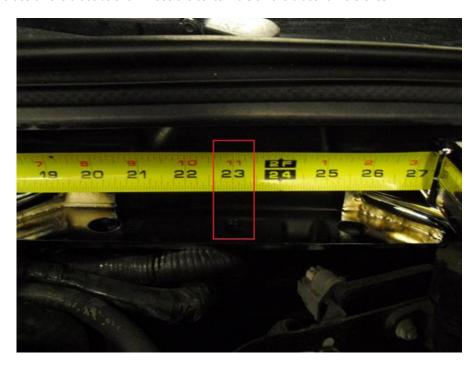
3. With brace properly aligned, carefully close the hood and make sure there is proper clearance. When you are certain that the brace is properly aligned and there is no interference when closing the hood, trace an outline of the rear of the brace onto the plastic firewall cover as shown. Make sure to push both down and back on the brace when tracing to ensure that it is resting on the firewall tab.
