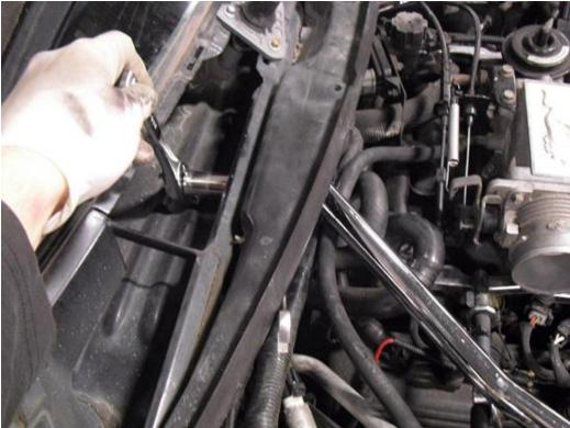
9. Once the brace is fully aligned and tightened, reinstall the rubber firewall molding, plastic cowl panel, and windshield wipers to complete the installation.
