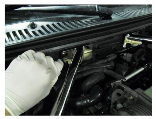
4. Remove the brace from the car. Remove the windshield wipers, rubber molding on firewall, and upper cowl panel. The plastic upper cowl is an extremely fragile piece so be very careful when removing it. Pull up with slight pressure between the windshield and panel and it should pop out easily. Before removing it completely, make sure to disconnect the washer lines.
