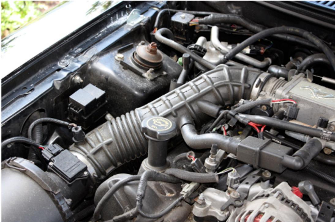
3. Remove the Throttle Cable, Cruise Control Cable and Throttle Body Spring from the left side of the throttle body. The throttle body spring simply unhooks from the throttle body. The Cruise Control Cable lifts straight "up" and pops off as pictured.
