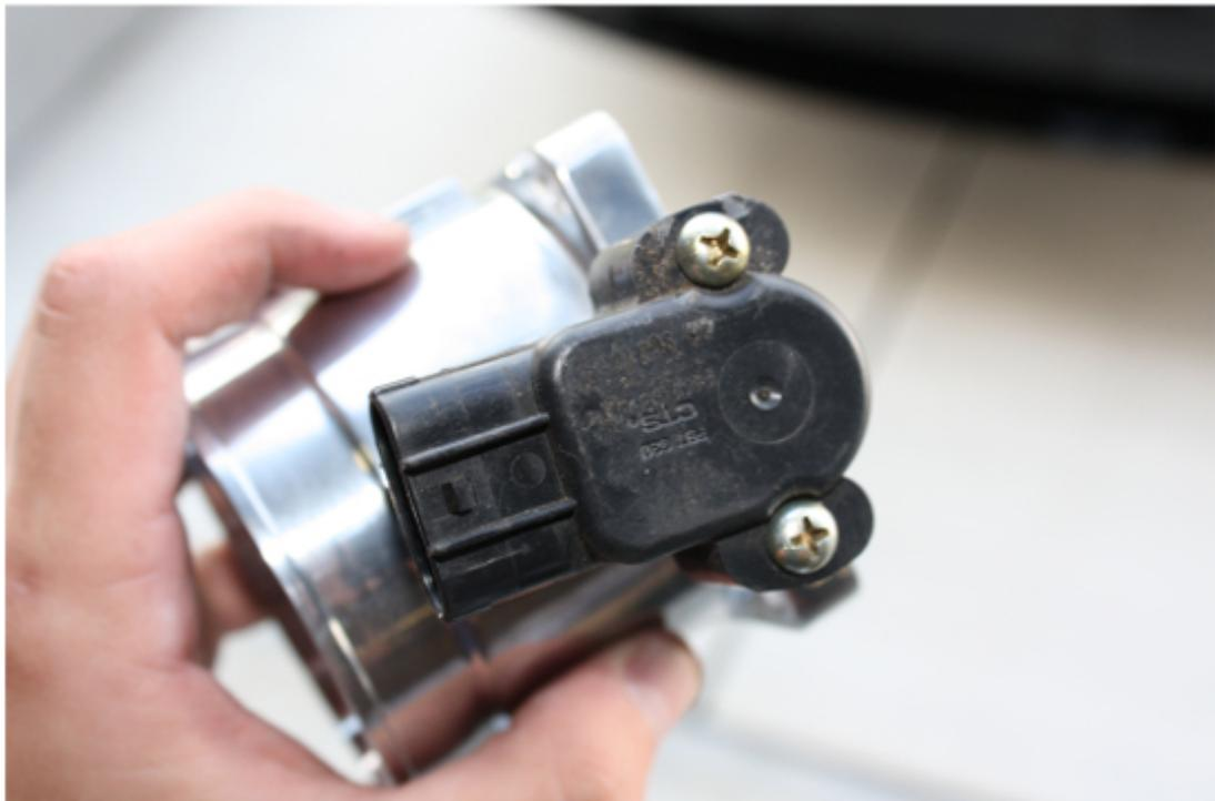
8. Install the stock Throttle Position Sensor onto your new Stack Racing Throttle Body. Using the included hardware, and the included gasket, bolt the new throttle body to the engine.
