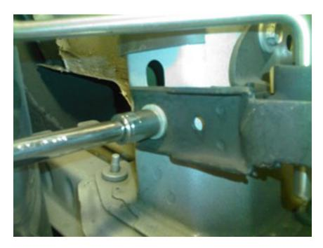
2. Now for the same bracket but for the top screw. For this step you will need to take the socket wrench extender off due to the lack of room to work in this area. With the extender off it is fairly easy to work. Turn counter clockwise loosening the bolt.
