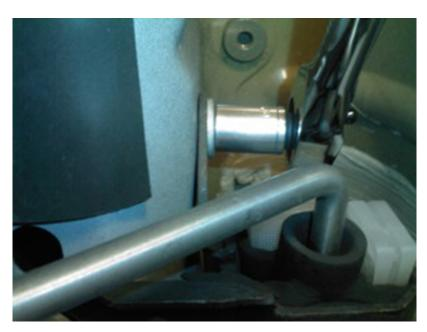
3. Now that both of the bolts have been taken off of the exhaust hanger you can work the hanger off of the exhaust bracket. You will need to grab it firmly and pull it while also working it back and forth to slip it off.
