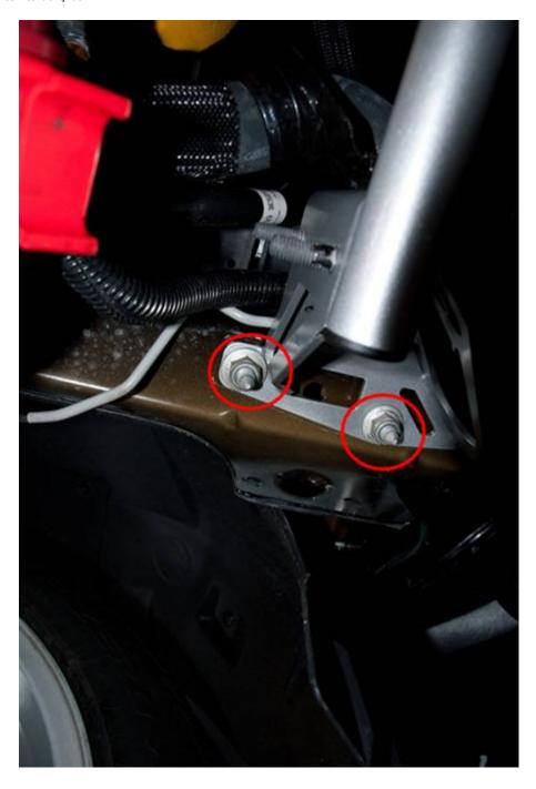
8. Secure the ac and brake lines to the support using the supplied zip ties, do not use all zip ties here as some will be used to secure your splashguards. Attach your sway bar to the support and tighten to 52 ft/lbs.
