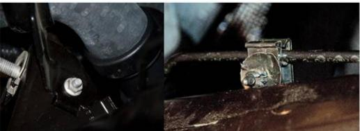
5. Support the radiator with your jack. Remove the 4 19mm nuts holding your stock radiator support. There are 2 nuts on the left and the right side of the support. Be careful as the stock support will fall after removing the last bolt.
