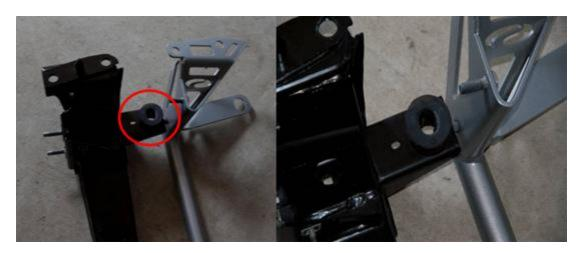
7. Install the Steeda Support and ensure the radiator bushings line up to the radiator pins. Reuse the stock 19mm nuts and tighten to 85ft/lbs.
