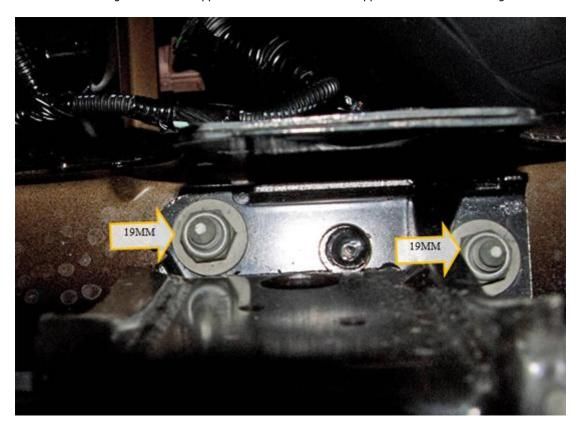
6. After removing the stock support from the car. Transfer over the radiator bushings from the stock support to the Steeda Radiator Support. The bushings are used to secure the radiator to the support. Please see pictures below for clarification.
