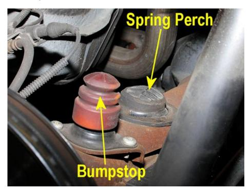
32. To install the new spring, simply place it into position. These particular springs do not have a certain orientation, so there is no "up" or "down". Note that they will be shorter than the factory springs, so there will be some gap that will be removed when you raise the rear axle back into position.
