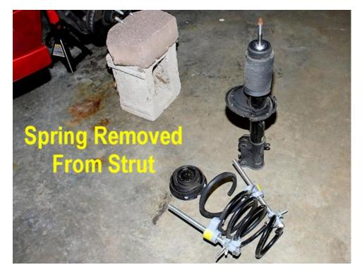
16. Reverse the turning direction of the spring compressors to expand them, switching between them every few turns. This will take a little longer than compressing them, as the strut already had them partially compressed and now they will be fully extending. Remove the compressors once the spring's tension has been fully released.
