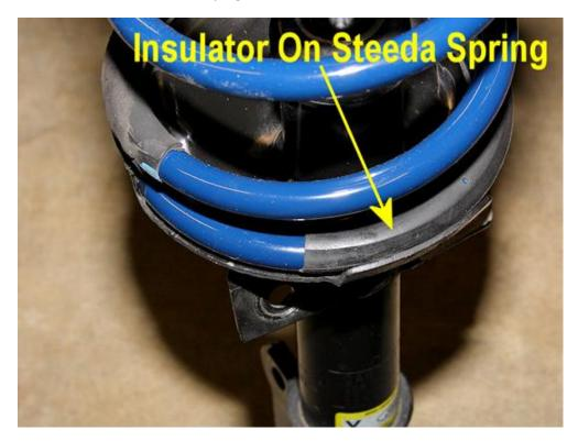
19. Install the spring compressors on the new spring, and then compress it. Since the Steeda Sport Springs are shorter than the stock springs, it doesn't take as much work to compress them for installation.
