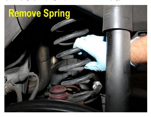
30. Take note of the upper spring perch/insulator. When reinstalling the spring, place the center of the perch inside the spring coils.
