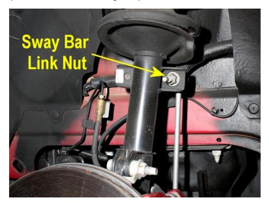
5. Use an 18mm wrench on the nut, and a 5/16 in. socket and socket wrench on the bolt. Hold the bolt still with the socket wrench while loosening the nut with the 18mm wrench. Once the sway bar is free, swing it out of the way.
