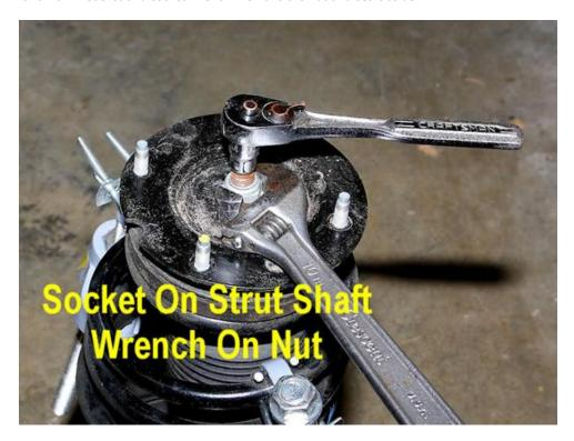
15. Disassemble the strut, by removing the upper plate, followed by the spring. Be careful with the upper plate, because it can separate which would result in the potential loss of the ball bearings located inside of it.
