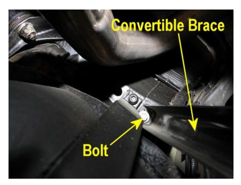
27. The image below provides a visual of what the brace looks like once it out of the car. There are 3 bolts located towards the front of the brace, two at the rear, and one for the bar in the middle. There are a total of two of these convertible braces you'll need to remove, one for each side of the car.
