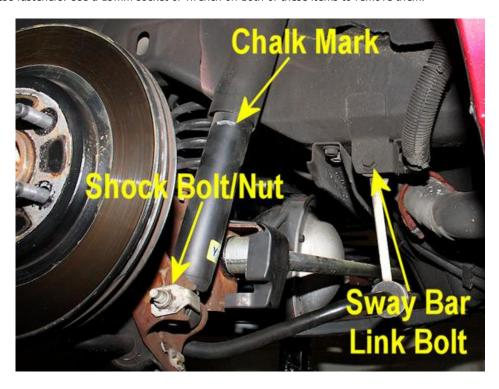
24. Turn the bottom of the shock so that it will clear its mount on the rear end when you lower it. Then swing the sway bar link out of the way as well.
