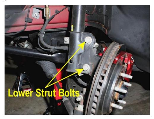
8. The lower strut bolts are tight. The use of a pipe or cheater bar to gain leverage is recommended. It will lessen the effort needed to break the bolt loose, and allow you to maintain better control of the socket wrench.
