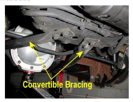
26. One of the bolts is located in the area directly in front of the rear axle. The brace has a long bar that reaches up into this area, and is home to the sixth bolt holding the brace in place. The sixth bolt has a smaller head than the other bolts, and you'll need to use a 13mm socket to remove it. A long socket extension will make this task much easier as well.
