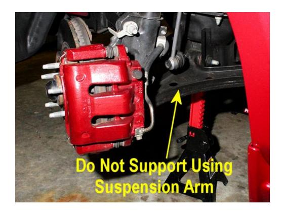
2. Next, raise the rear of the vehicle, and support it with jack stands paced in front of the rear axle close to the side jacking points. You do not want to support the car by the rear axle, as you will be lowering the axle. For now, support the axle with a jack under the center of the housing. Remove the rear wheels, and set them aside.
