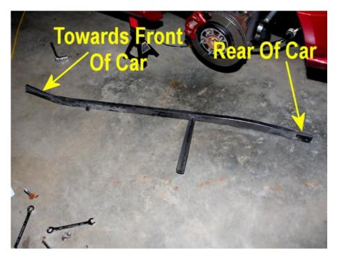
28. With the convertible bracing removed, if you have a convertible, it's now time to lower the rear axle. Using the jack, slowly lower the rear axle as far as it will go. Notice that the panhard bar, stock or otherwise can remain attached.
