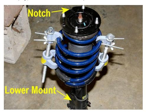
20. Use the strut's nut as a reference point to determine if you have compressed the spring enough for installation. While the factory rust at the top of the strut is an eyesore, this is one time it comes in handy. It'll let you know how far down the nut was threaded previously, and whether you've compressed the Steeda spring enough for reinstallation.
