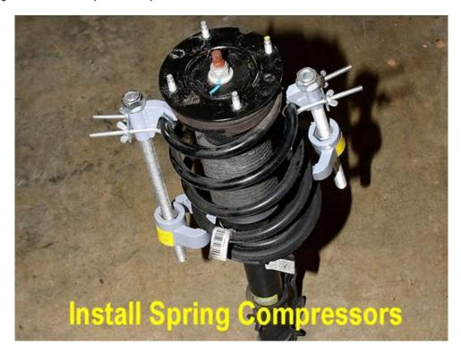
13. Once the spring pulls away from the top and the bottom of its resting position on the strut, and a gap forms, the spring has been compressed enough to disassemble the strut. You don't have to fully compress the strut, just simply compress it enough that there is no tension against the upper or lower plates.
