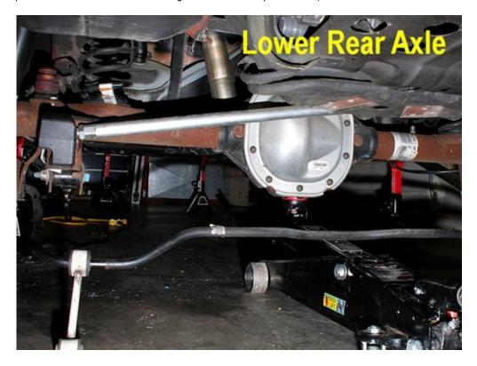
29. Once you've lowered the axle, you should be able to remove the rear springs with a slight amount of effort. You'll have to pull up on the spring as you are pulling it out, so that it will clear the lower spring perch.
