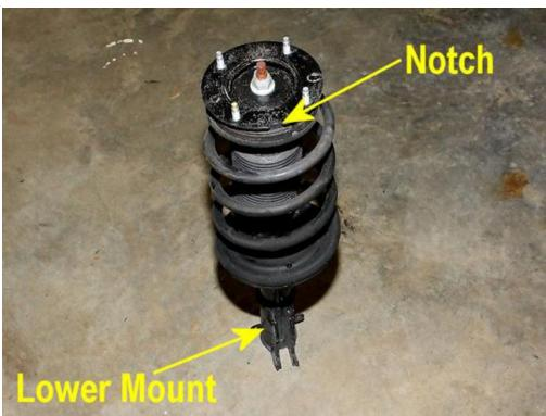
12. Install your spring compressors, as shown in the directions that accompany them. Carefully compress the springs, alternating between each compressor every few turns.
