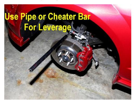
9. Once the lower strut bolts are removed, the suspension arm will fall free. Support it with something similar to a jack stand or a cinder block. Be careful not to damage the threads on the wheel studs when doing so.
