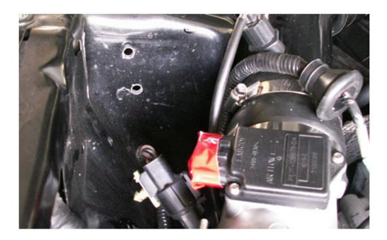
10. Put the brace back into the car and bolt it down with the hardware from the kit. Use a 1/2 " wrench and 1/2 " socket (3/8" or 1/2 " drive) to tighten the bolts. Use a jack and a stand for safety to lift one side of the car at a time, in order to get the nuts started and tightened for the bolts on the strut tower.
