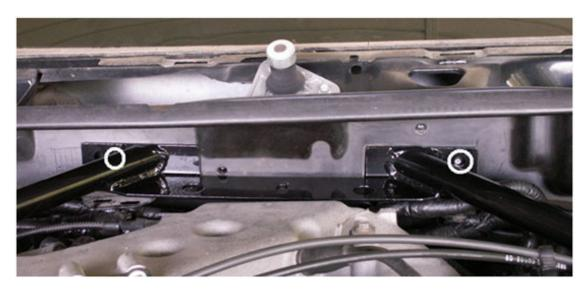
9. Remove the brace and drill the holes using a 5/16" drill bit. Using a punch will help keep the drill bit from walking You may need to take the intake off the car to drill the holes on the side of the passenger strut tower on some Mustangs with stock air intakes. This will require a 5/16" socket/wrench and a flat head screwdriver. Make sure to tape up any sensors you unplug or the throttle body, if you remove the air intake, to keep shavings out of the engine.
