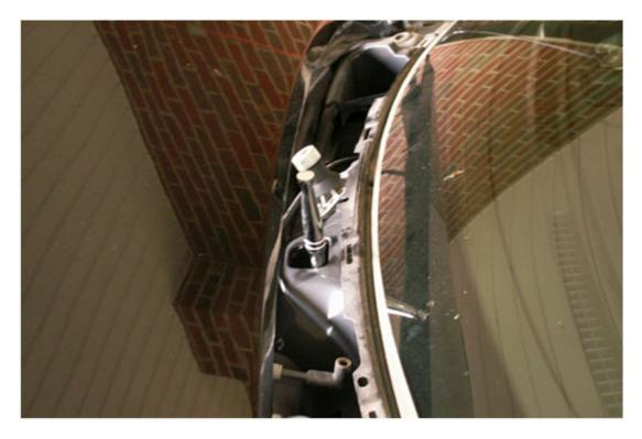
11. Put the plastic cowl panel back on. Snap the push pins back into place and put the rubber strip back on the plastic firewall panel. Put the windshield wipers back on to complete the installation.
