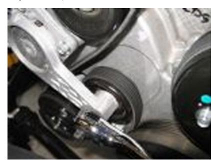
5. Maintaining pressure on the tensioner, slide the belt off the water pump pulley and then remove it from the engine bay, making sure not to put any tears or rips in the belt.
