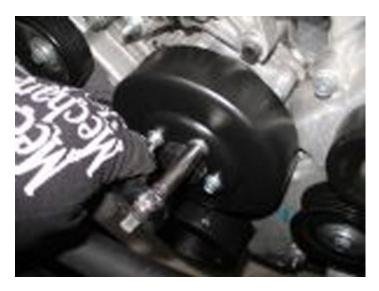
15. Install the new water pump pulley. Tighten these bolts to 18 ft-lbs. of torque. **Note:** These are the bolts that were set aside in Step 6.
