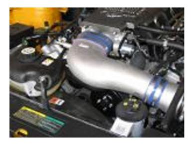
17. Reinstall the air intake tube (In reverse order of removal). Next, start the vehicle to ensure that the accessory belt tracks correctly, and there is no rubbing.
