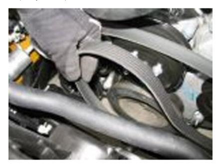
6. Remove the retainer bolts for the water pump pulley and then remove the pulley from the water pump. **Note:** Set the retainer bolts for the water pump aside, as they are re-used to install the new Steeda water pump pulley.
