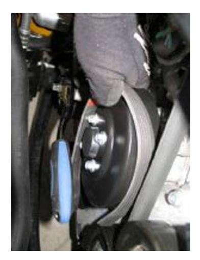
16. Reinstall the accessory belt, using the factory routing, once again being careful not to damage the belt in anyway.
