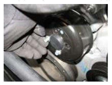
7. With the water pump pulley removed, loosen the alternator's lower right retainer nut and remove the stud. A 7mm socket or wrench is required to remove the stud.
