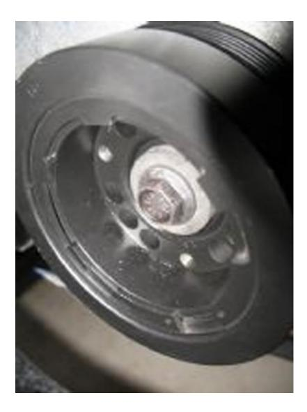
13. Align the key slot of the pulley to the key of the crank shaft and use the longer bolt supplied with the underdrive kit to pull the new pulley into place on the crankshaft. Once the pulley is sufficiently on the shaft, remove the longer bolt and replace it with the shorter bolt supplied in the kit to finish pulling the pulley into place. **Caution:** Do **NOT** tighten the longer bolt all the way as damage can occur to the crank shaft.
