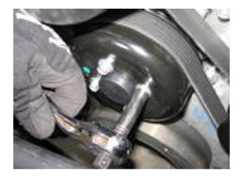
4. Using a 1/2" socket driver or breaker bar, apply downward force on the belt tensioner to release the pressure on the accessory belt. Doing this will relieve pressure off the belt and allow for its removal.
