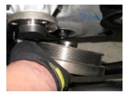
11. Remove the crank pulley from the vehicle.
