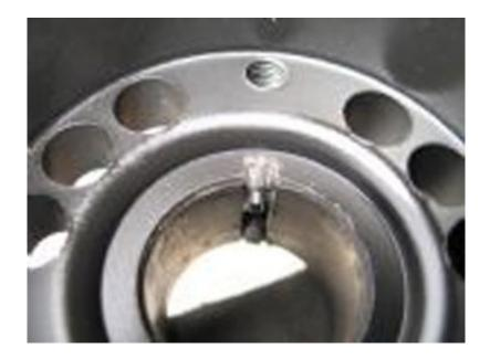
12. Prior to installing Steeda's underdrive crank pulley, apply a dab of high temperature silicone sealer (gasket maker) to the key slot. This step ensures that oil cannot come out while installing the underdrive pulley.
