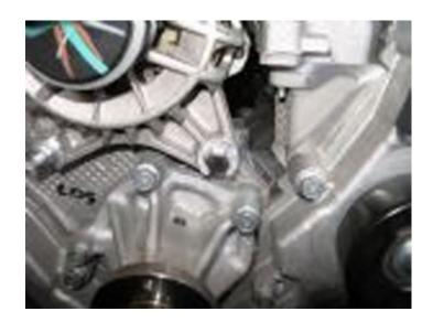
9. Using a three prong puller, start removing the crank pulley from the crank shaft. Using this tool is quite simple. Screw the tool onto the crankshaft and tighten the nut as much as possible by hand. Then just hold the end of the tool with a wrench and use another wrench to tighten the larger nut.
