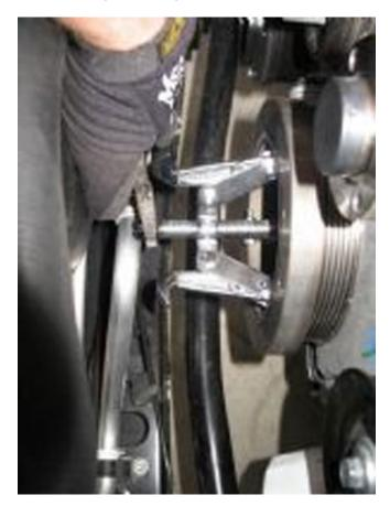
10. Verify that your three pronged puller is positioned properly on the crank pulley. This will ensure nothing is damaged during the pulley removal process. An alternate method of installing the crankshaft pulley is recommended by Steeda. They recommend the torque turn method. Steeda claims it is more accurate. The torque turn measures how much the bolt is stretched which is really what is desired. Friction from the bolt head and washer is a factor which leads to inaccurate torque of a fastener.
