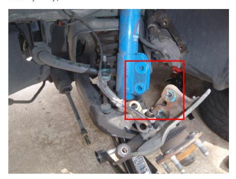
7. Continue with the driver's side, and disconnect the sway bar end link nut. This nut is also 15mm in size but you will need a deep socket. If you just remove the top nut and top bushing, that is enough.
