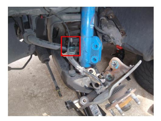
8. Finally, if your car has ABS, you need to remove the ABS sensor from the spindle using a ¼" 6-point socket. I used a 12-point, which also works fine. Once removed, lay the sensor on top of the caliper where it is out of the way.
