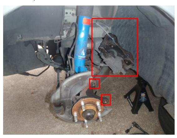
5. Next, straighten and remove the cotter pin that goes through the castle nut that attaches the tie-rod. Then use an 18mm deep socket and remove the castle nut itself. Now the tierod can fall out of the spindle, however, it may require some persuasion. If it doesn't come out on its own, first, spray it with penetrating fluid. Let it sit for a few minutes and then hit the top of the bolt with a hammer to force it out.
